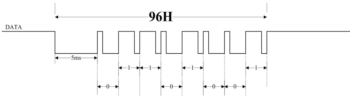
If we want the chip to play the voice content of address 01/02/03/04 in sequence. That is, the code-linking command playback, F3+01+F3+02+F3+03+F3+04. The corresponding sequence diagram can be shown as
