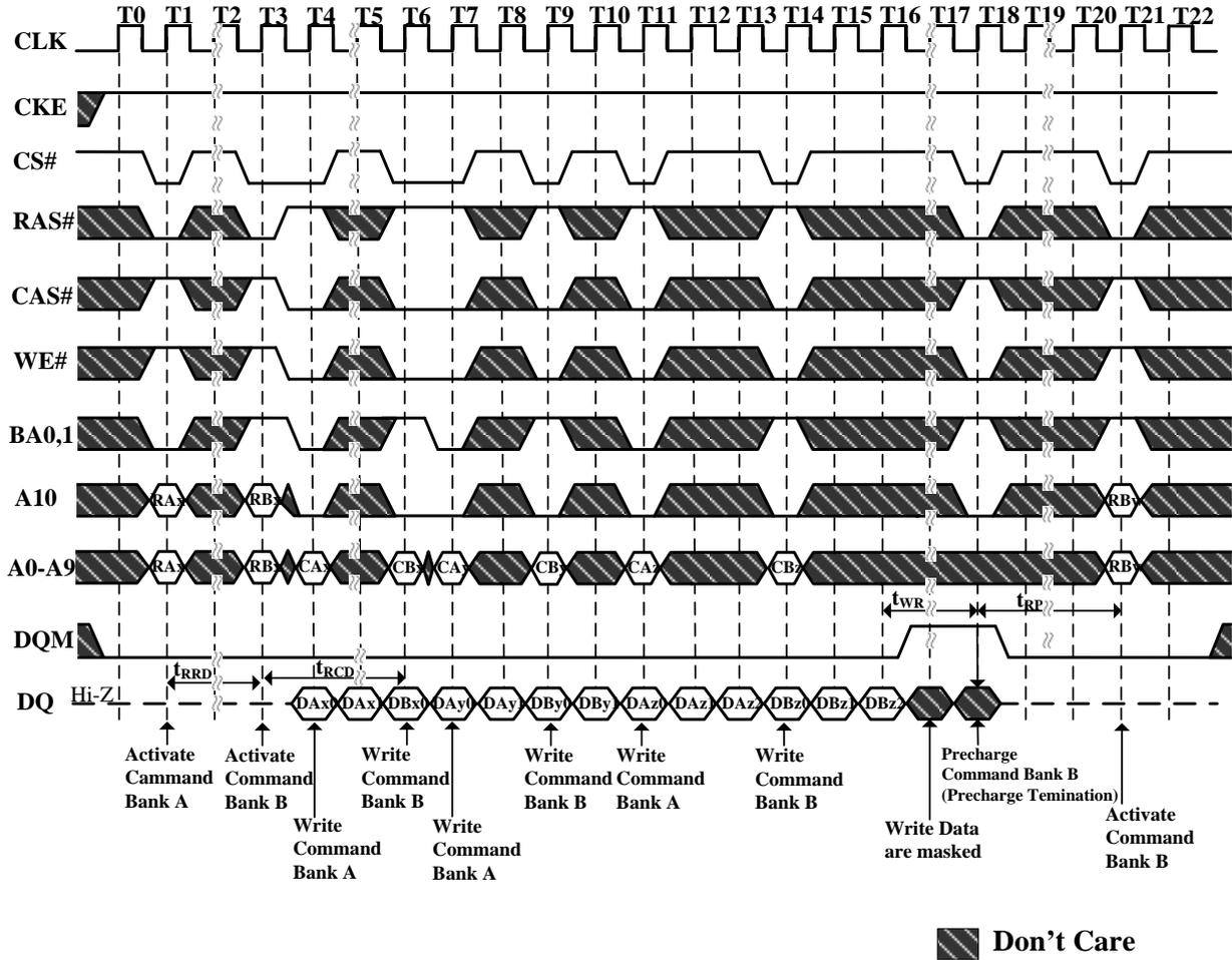
**Figure 42. Precharge Termination of a Burst**
