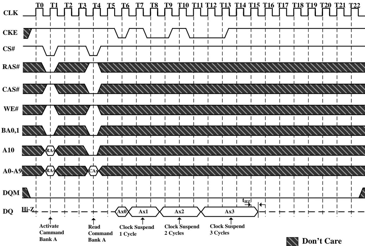
**Figure 24.2. Clock Suspension During Burst Read (Using CKE)**
