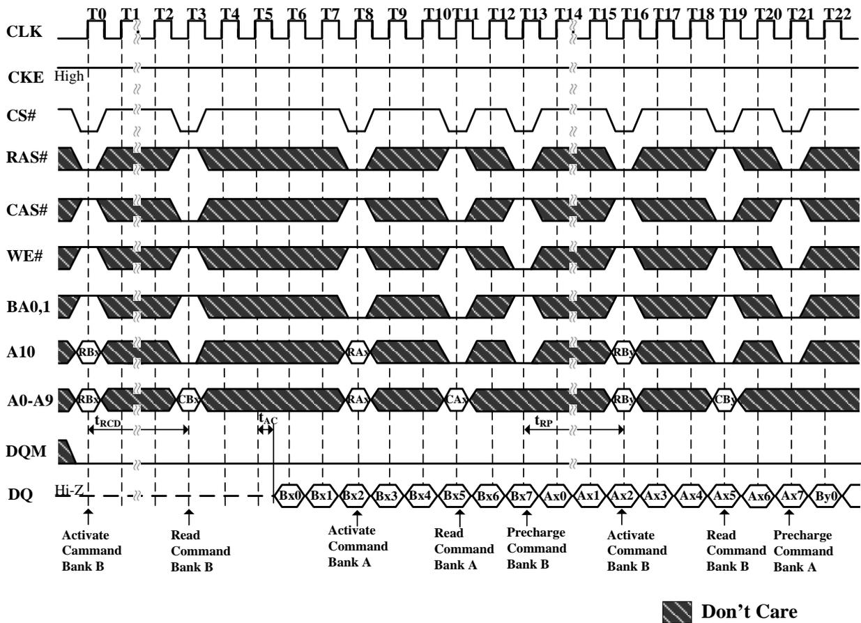
**Figure 30. Random Row Write (Interleaving Banks)**
