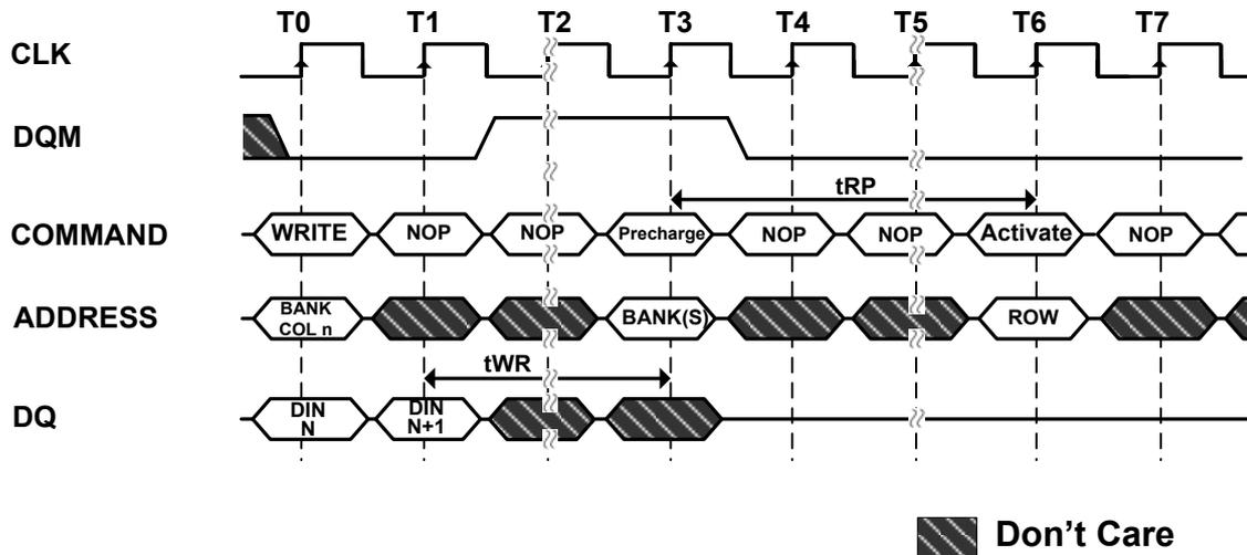
**Note:** The DQMs can remain low in this example if the length of the write burst is 1 or 2.
