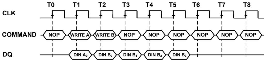
The Read command that interrupts a write burst without auto precharge function should be issued one cycle after the clock edge in which the last data-in element is registered. In order to avoid data contention, input data must be removed from the DQs at least one clock cycle before the first read data appears on the outputs (refer to the following figure). Once the Read command is registered, the data inputs will be ignored and writes will not be executed.
