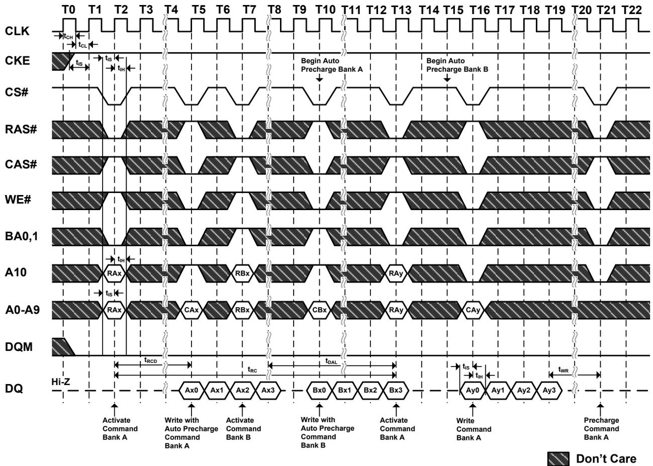
**Figure 20. AC Parameters for Read Timing (Burst Length=2, CAS# Latency=2)**
