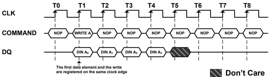
A write burst without the auto precharge function may be interrupted by a subsequent Write, BankPrecharge/PrechargeAll, or Read command before the end of the burst length. An interrupt coming from Write command can occur on any clock cycle following the previous Write command (refer to the following figure).
