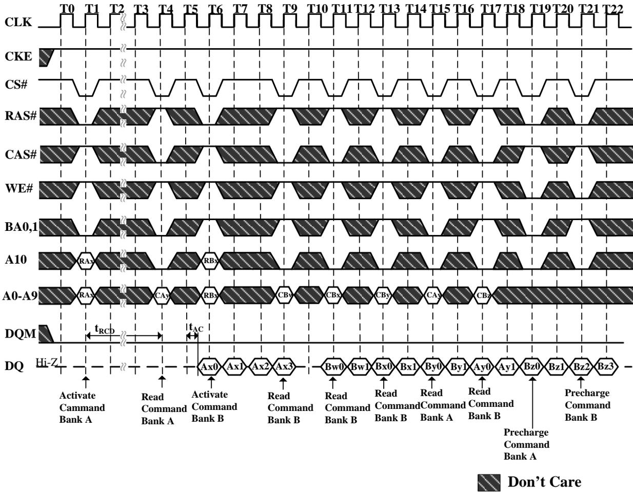
**Figure 32.2. Interleaved Column Read Cycle (Burst Length=4, CAS# Latency=3)**
