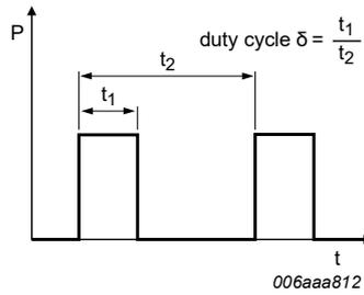
Fig. 17. Duty cycle definition
