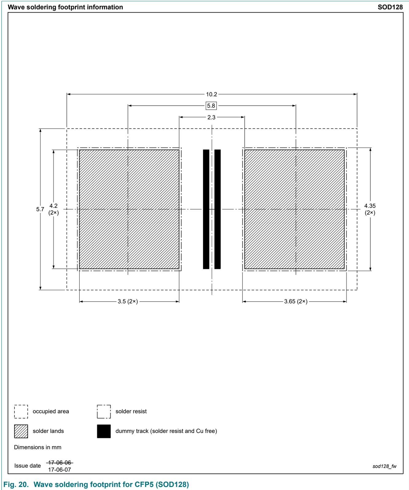
**Fig. 20. Wave soldering footprint for CFP5 (SOD128)**
