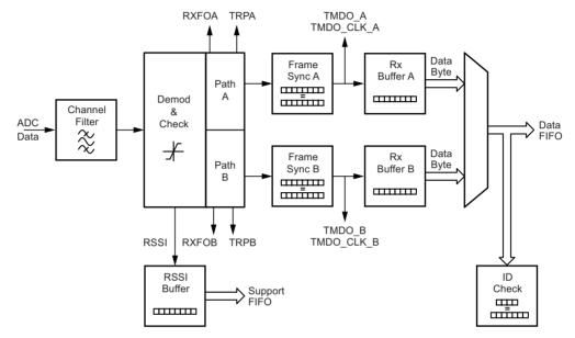
The channel filter determines the receiver bandwidth. Its output is used for both receiving paths A and B, making it necessary to configure the filter to match both paths. The receiving paths A and B are identical and consist of an ASK/FSK demodulator with attached signal checks, a frame synchronizer which supports pattern-based searches for the telegram start and a 1-byte hardware buffer with integrated CRC checker for the received data.
