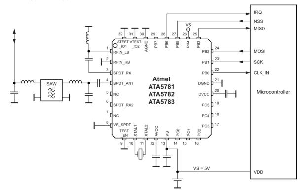
Figure 1-3 shows a typical vehicle side application circuit with an external host microcontroller running from a 5V voltage regulator. The pin PB4 (PWRON) is directly connected to VS and the Atmel<sup>®</sup> ATA5781/2/3 enters the IDLEMode after power-on. In this configuration the Atmel ATA5781/2/3 can work autonomously and the microcontroller stays powered down to keep current consumption low while remaining sensitive to RF telegrams.
