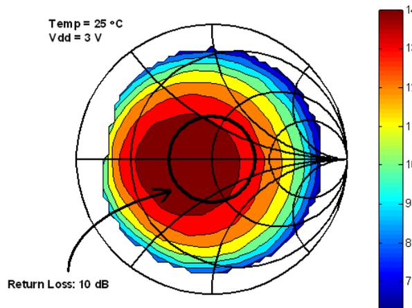
**Figure 4-17. Output Power vs Load Impedance (+14-dBm Setting)**
