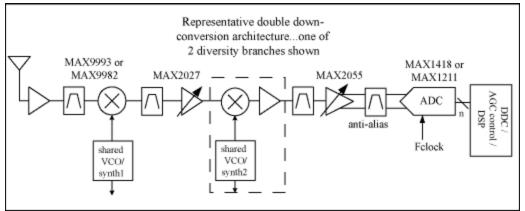
Figure 1. Subsampling receiver architecture.
