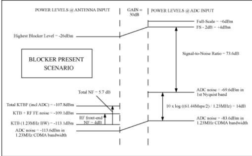
Figure 3. ADC noise contribution for blocker present. MAX1211 Allows Single Down Conversion Architecture
