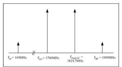
Figure 4. Frequency locations for desired f<sub>RF</sub>, f<sub>LO</sub>, f<sub>IF</sub>, and undesired f<sub>Half-IF</sub>.
