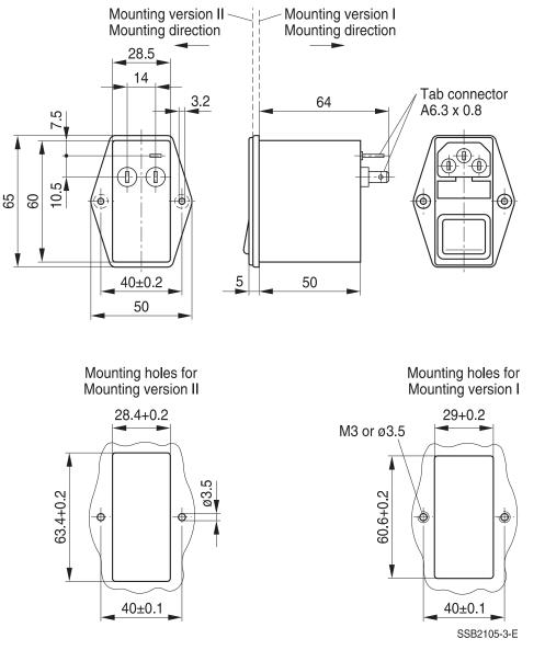
General tolerances according to ISO 2768-cL Dimensions in mm
