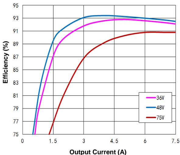
Figure 1. Efficiency vs. Load Current (25 $^\circ C$ )
