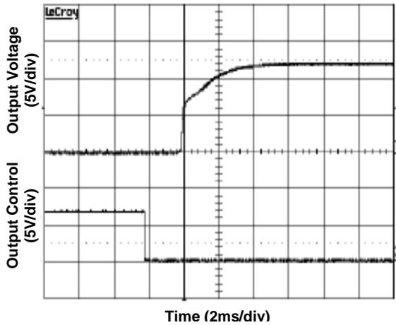
Figure 3. Start-Up from Enable Control
