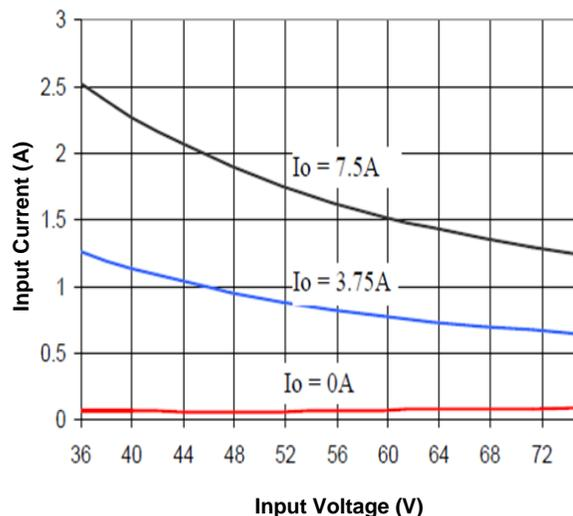
Figure 2. Input Characteristics
