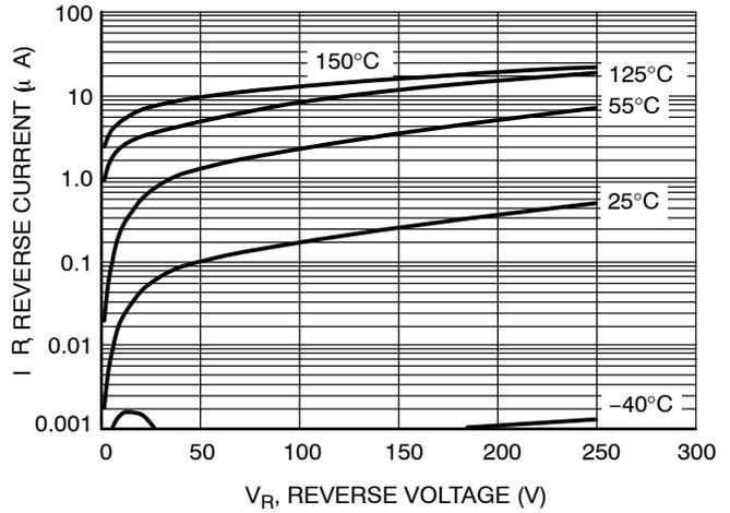
**Figure 3. Leakage Current**
