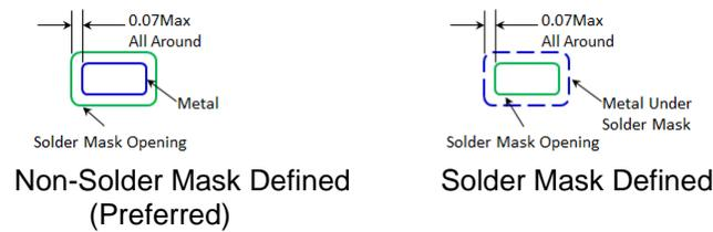
**Figure 10 Solder Mask Pattern**
