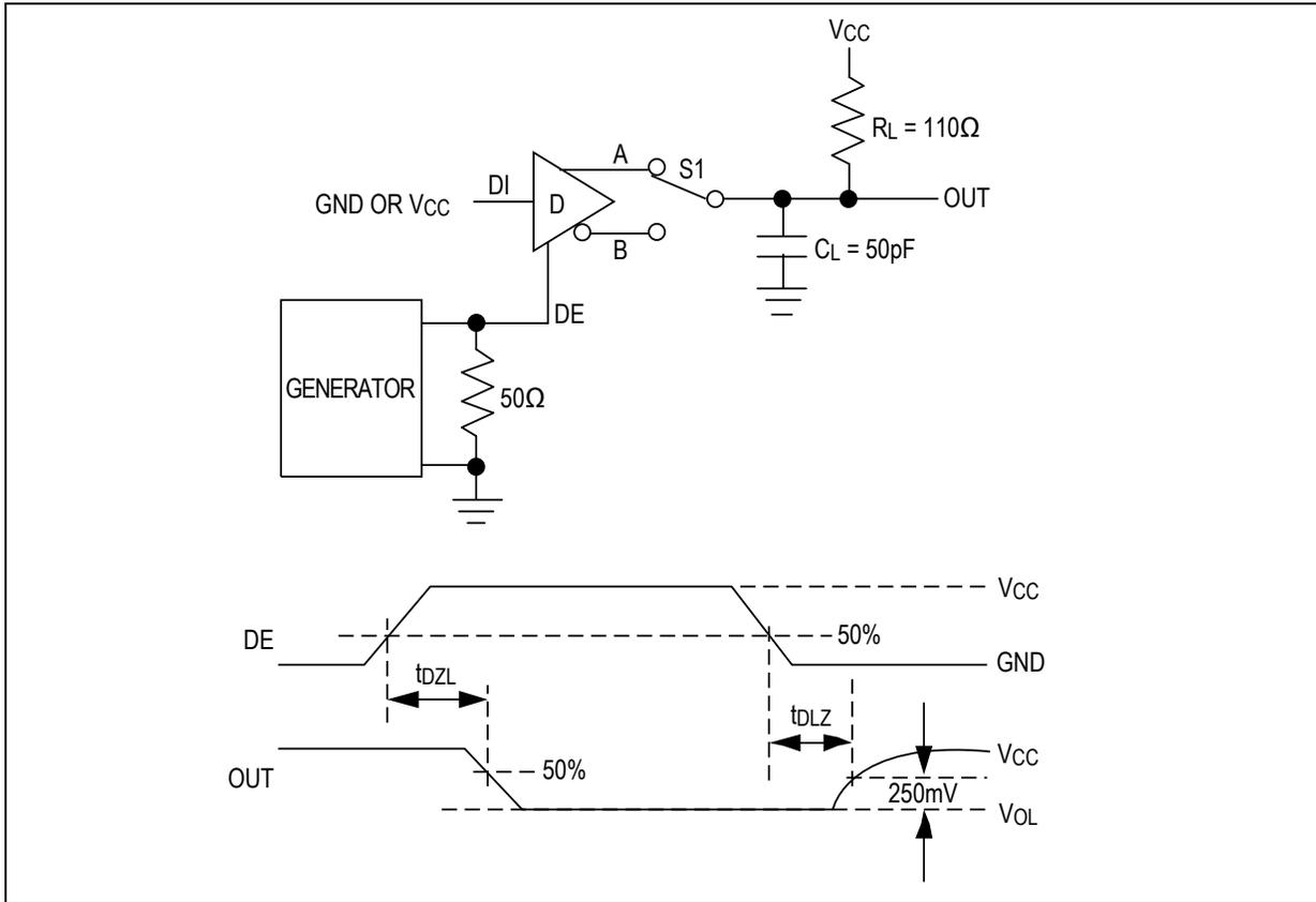
Figure 5. Driver Enable and Disable Times ( $t_{DZL}$ ,  $t_{DLZ}$ )
