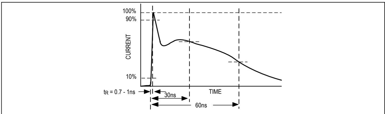
Figure 12. IEC 61000-4-2 ESD Generator Current Waveform
