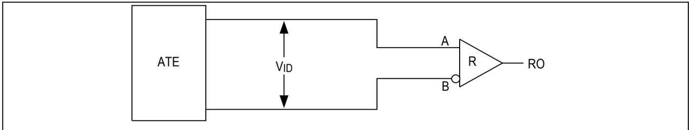
Figure 6. Receiver Propagation Delay Test Circuit
