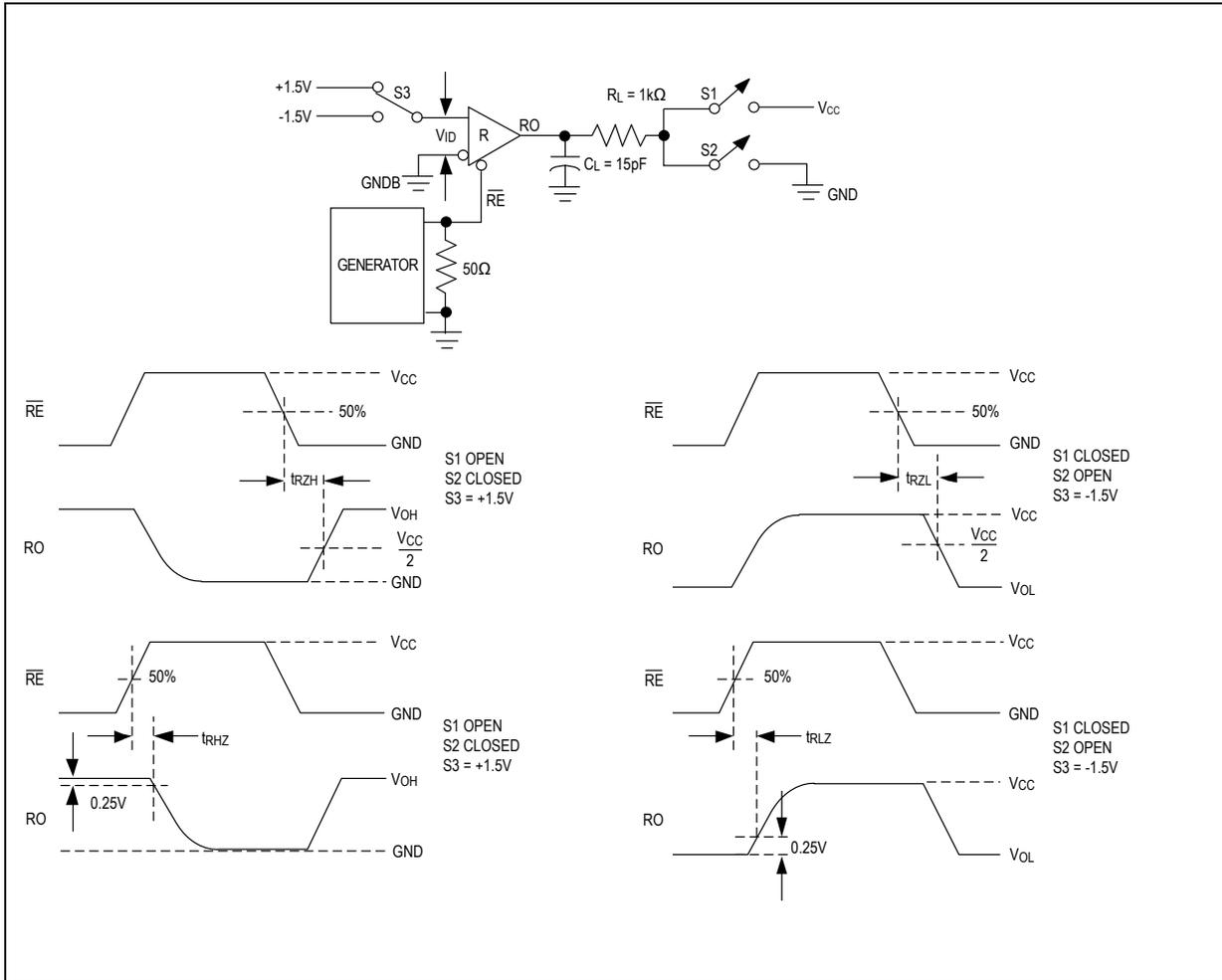
Figure 8. Receiver Enable and Disable Times
