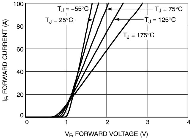
Figure 1. Forward Characteristics
