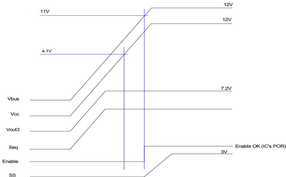
Fig. 3: Normal Start up, Enable threshold is externally set to 11V
