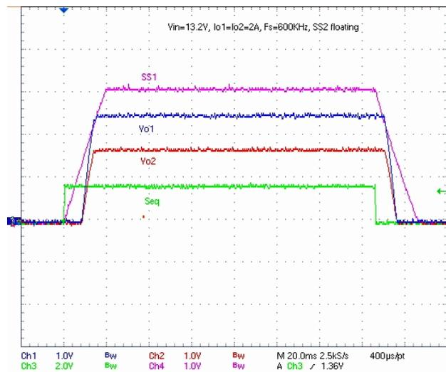
Fig. 10: Ratiometric Power Up / down
