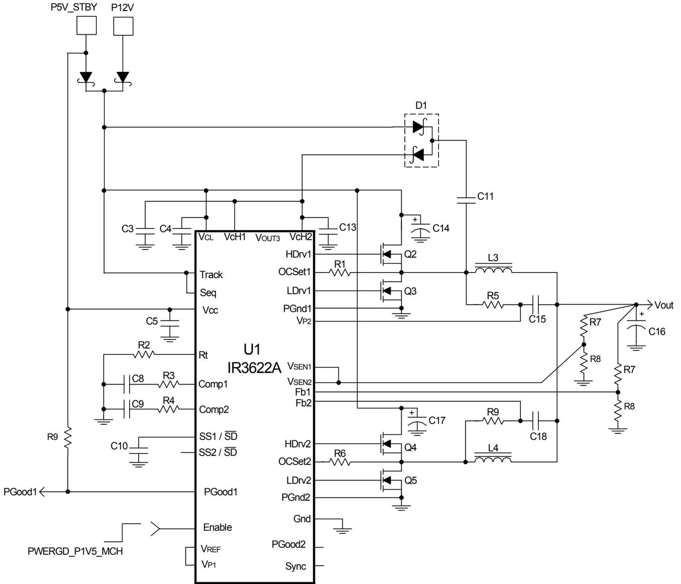
Fig. 25: Application circuit for FBD P1V8 VREG(40A)
