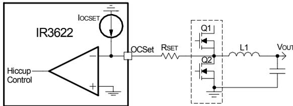
Fig. 13: Connection of over current sensing resistor
