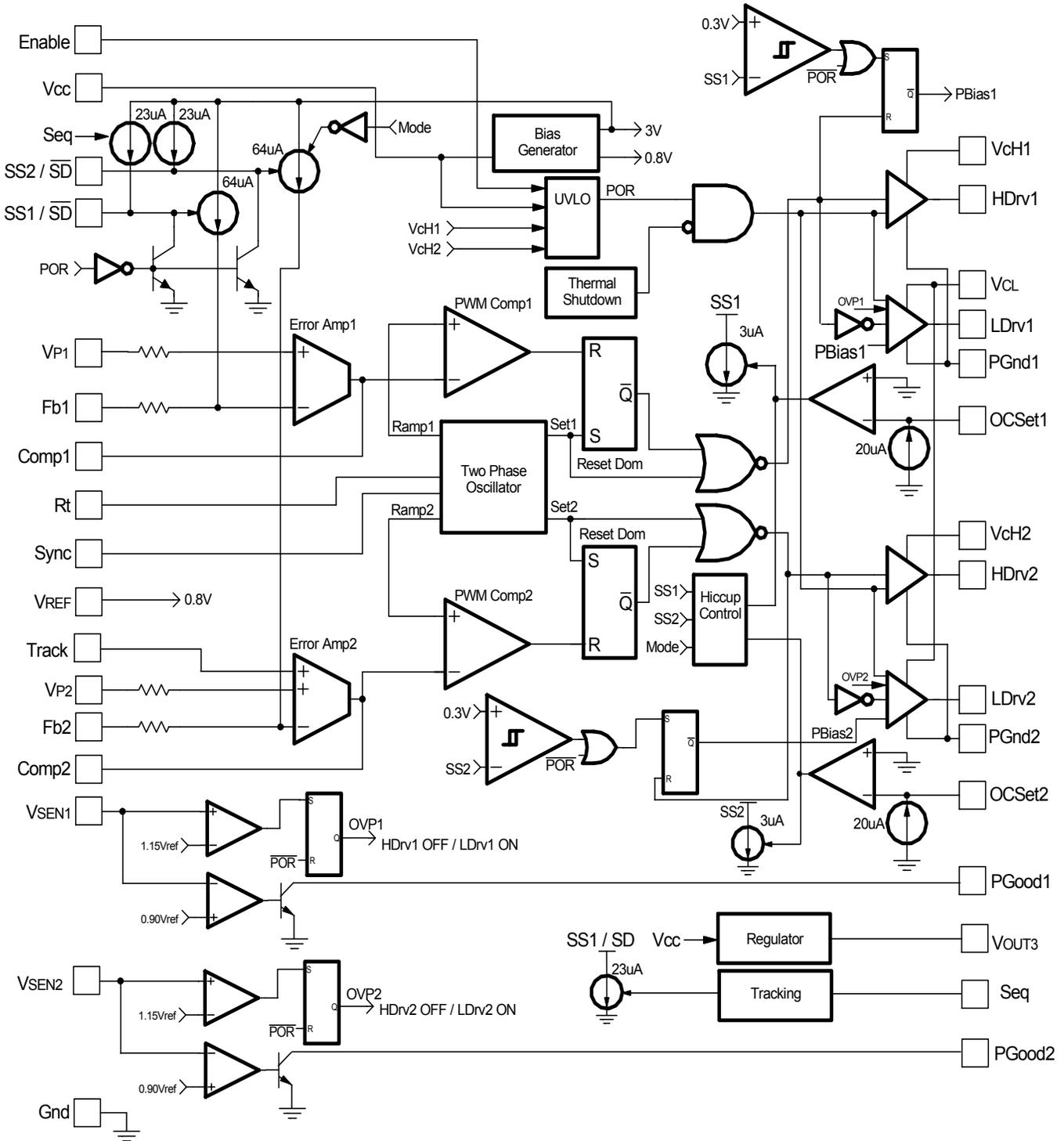
Fig. 2: Simplified block diagram of the IR3622A
