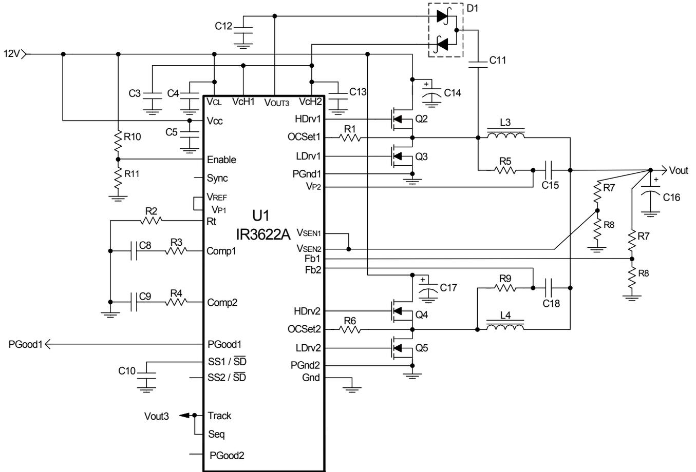
Fig. 23: Application circuit for 12V to 1.8V @ 40A
