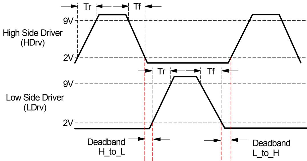
Fig. 1: Rise / Fall and deadband time for driver section
