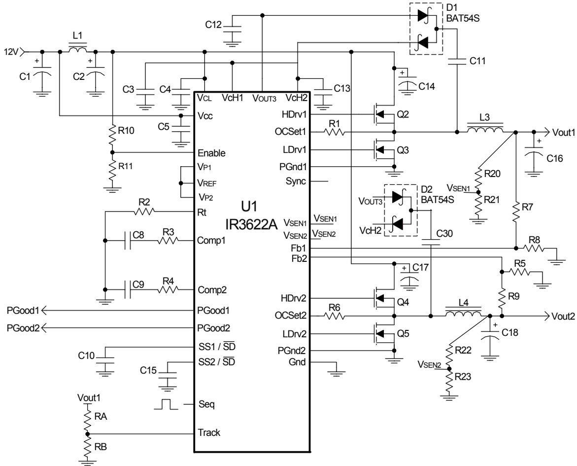
Fig. 24: Application circuit for Dual output application
