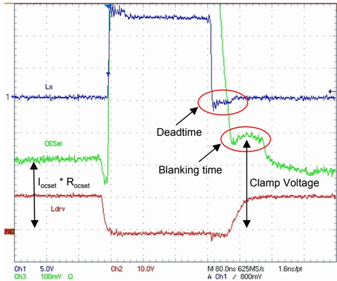
Fig. 15: OCset pin during normal condition
