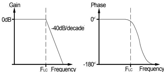
Fig. 19: Gain and Phase of LC filter
