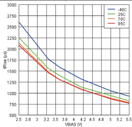
Figure 22. V<sub>BIAS</sub> vs t<sub>R</sub> (V<sub>IN</sub> = 2.5 V, C<sub>T</sub> = 1 nF)
