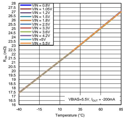
Figure 6. Temperature vs  $R_{ON}$  ( $V_{BIAS} = 5.5 V$ )
