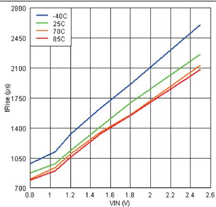
Figure 20. V<sub>IN</sub> vs t<sub>R</sub> (V<sub>BIAS</sub> = 2.5 V, C<sub>T</sub> = 1 nF)
