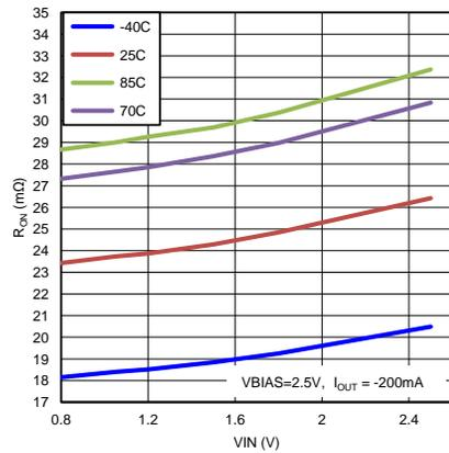
Figure 7.  $V_{IN}$  vs  $R_{ON}$  ( $V_{BIAS} = 2.5 V$ )
