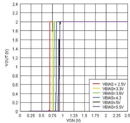
Figure 11.  $V_{ON}$  vs  $V_{OUT}$  ( $T_A = 25^\circ\text{C}$ )
