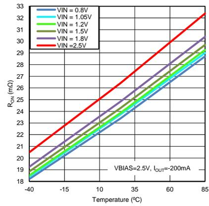
Figure 5. Temperature vs  $R_{ON}$  ( $V_{BIAS} = 2.5 V$ )
