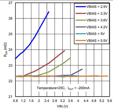
Figure 9.  $V_{IN}$  vs  $R_{ON}$  ( $T_A = 25^\circ\text{C}$ )
