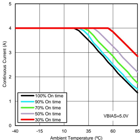
*On time* is the duration of time that the device is enabled ( $ON \geq V_{IH}$ ) over 70,000 hour lifetime.
