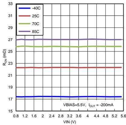
Figure 8.  $V_{IN}$  vs  $R_{ON}$  ( $V_{BIAS} = 5.5\text{ V}$ )
