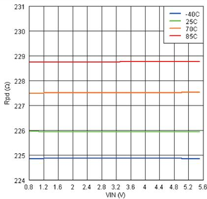
Figure 10.  $V_{IN}$  vs  $R_{PD}$  ( $V_{BIAS} = 5.5\text{ V}$ )
