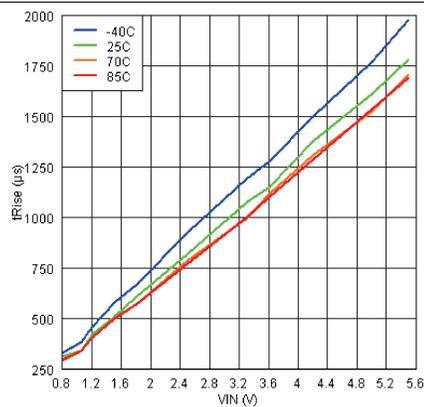
Figure 21. V<sub>IN</sub> vs t<sub>R</sub> (V<sub>BIAS</sub> = 5.5 V, C<sub>T</sub> = 1 nF)
