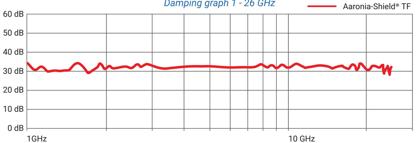
Damping specifications for Aaronia SHIELD® TF shielding foil
