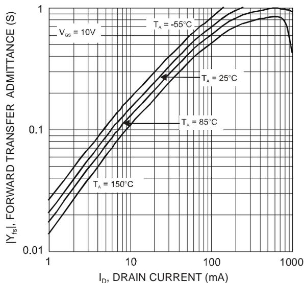
Fig. 11 Forward Transfer Admittance vs. Drain Current
