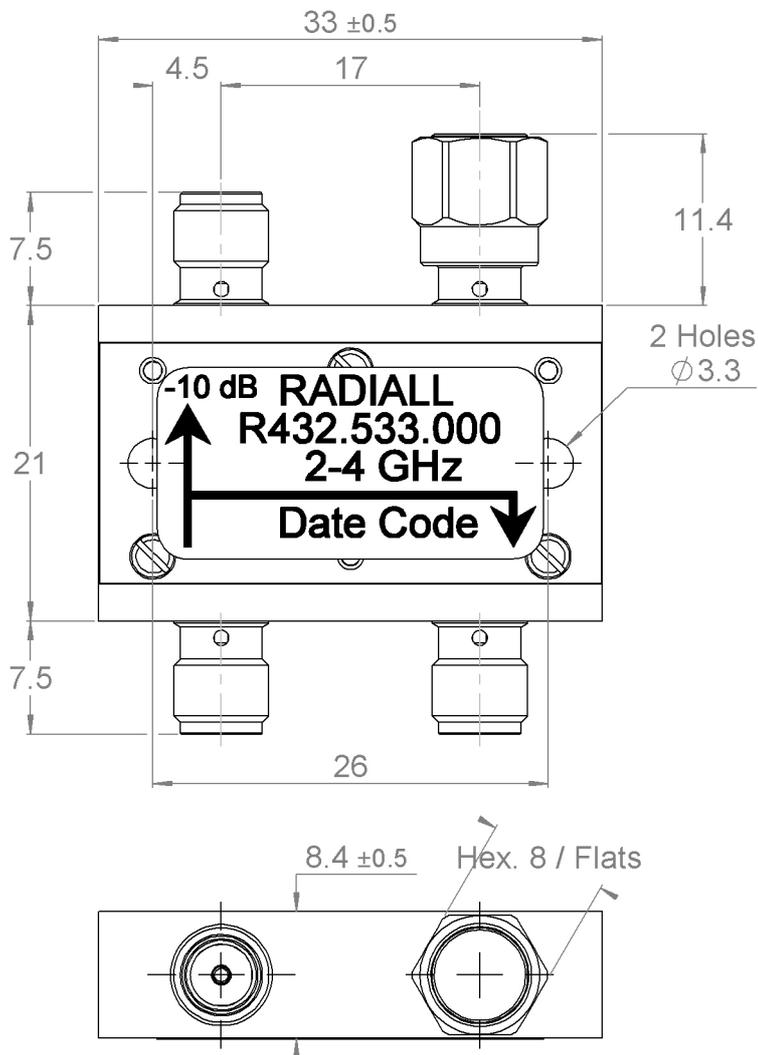
All dimensions are in mm. Tolerances according ISO 2768 m-H
