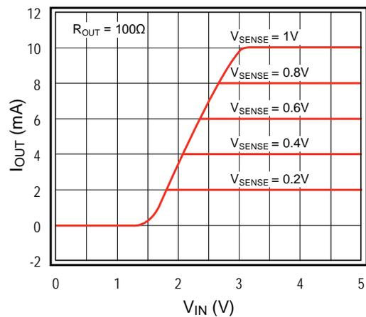
**Figure 9. Transfer Characteristics**
