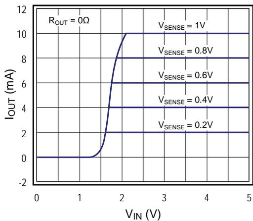
**Figure 8. Transfer Characteristics**
