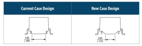
In addition, the marking appearance of the transformer will be changed to be consistent with similar product types. This marking change will have no effect on the fit, function, quality or reliability. The product's form will change slightly due to the marking format modification.
