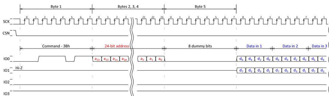
Figure 90: 24-bit READ2O (dual-read output), SPI MODE = MODE0
