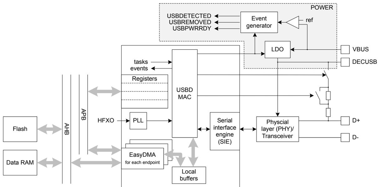
Figure 195: USB device block diagram
