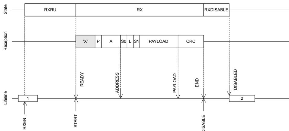
Figure 117: Receive sequence using shortcuts to avoid delays
