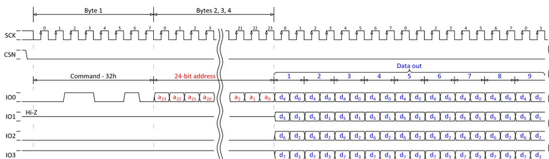
Figure 96: 24-bit PP40 (quad page program output), SPI MODE = MODE0
