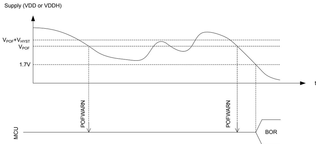
Figure 20: Power-fail comparator (BOR = brownout reset)
