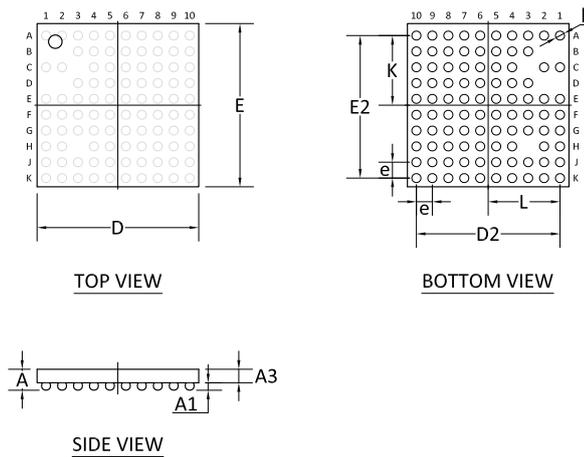
Figure 212: WLCSP 3.544 x 3.607 mm package
