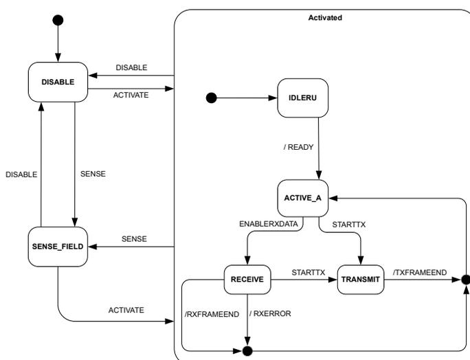
Figure 64: NFCT state diagram, automatic collision resolution disabled
