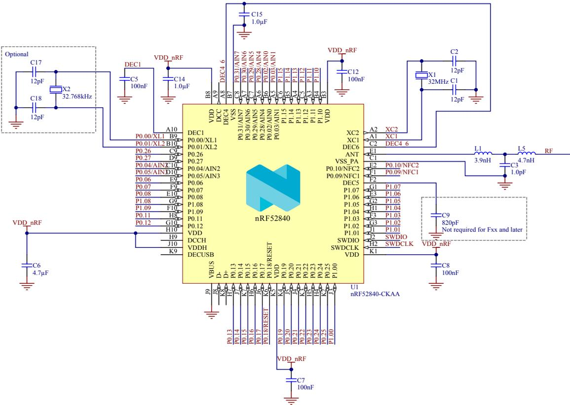
Figure 226: Circuit configuration no. 6 schematic for CKAA WLCSP
