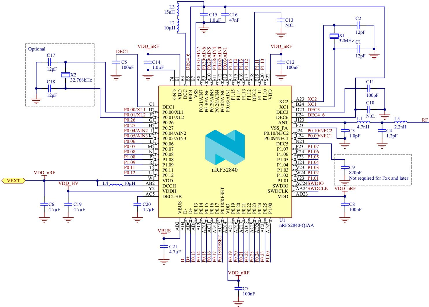
Figure 219: Circuit configuration no. 7 schematic for QIAA aQFN™ 73
