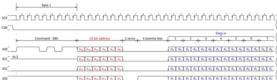
Figure 93: 24-bit READ4IO (quad-read input/output), SPIMODE = MODE0
