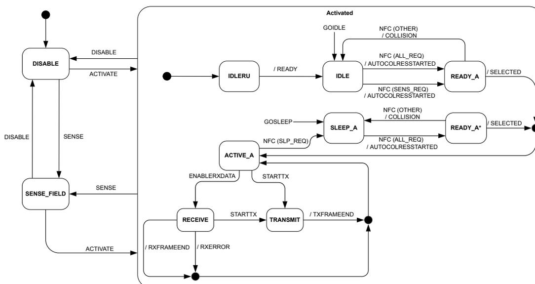
Figure 63: NFCT state diagram, automatic collision resolution enabled
