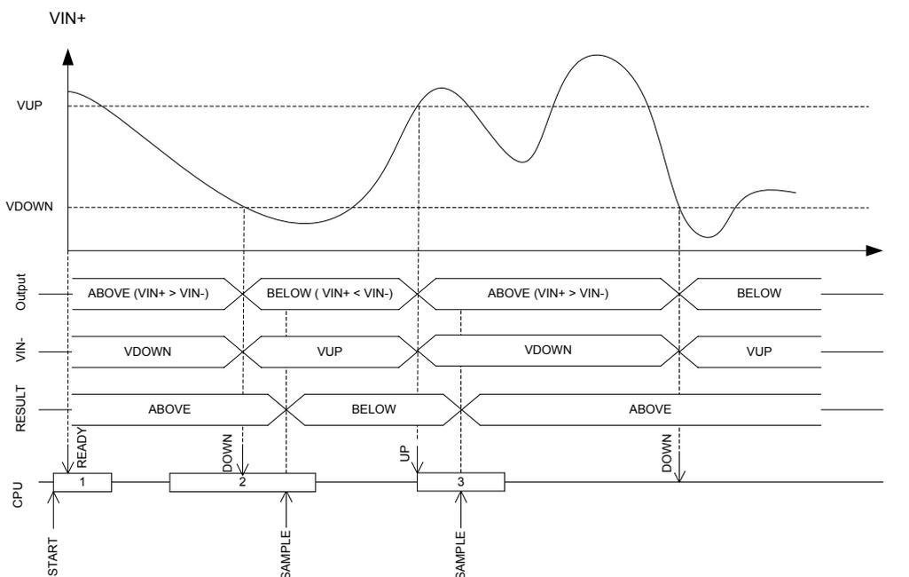
Figure 43: Hysteresis example where  $VIN+$  starts above **VUP**
