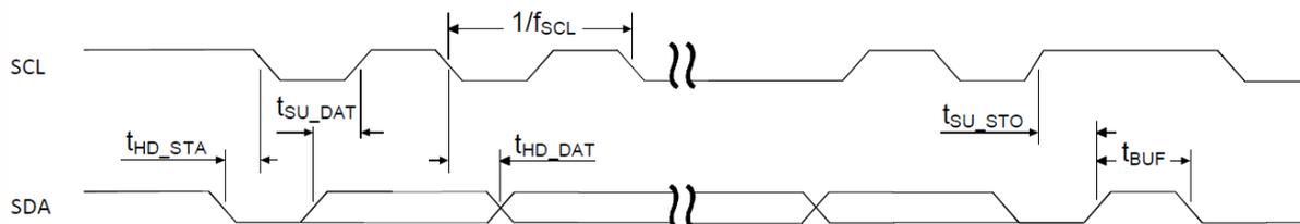
Figure 171: TWI timing diagram, 1 byte transaction
