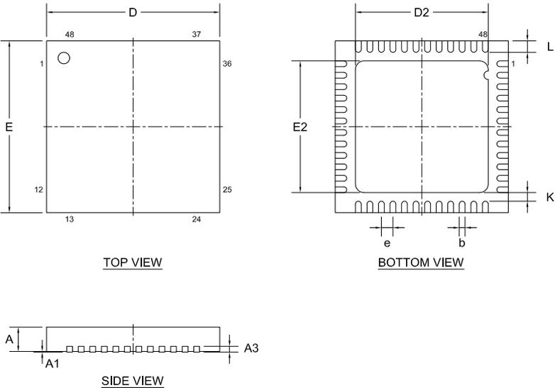
Figure 211: QFN48 6 x 6 mm package
