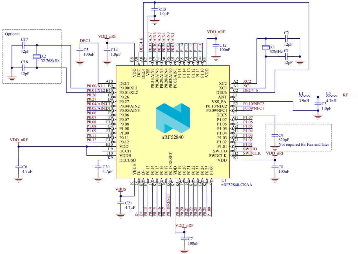
Figure 223: Circuit configuration no. 3 schematic for CKAA WLCSF
