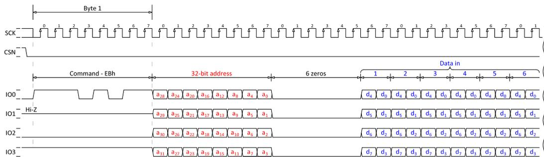
Figure 102: 32-bit READ4IO (quad-read input/output), SPIMODE = MODE0
