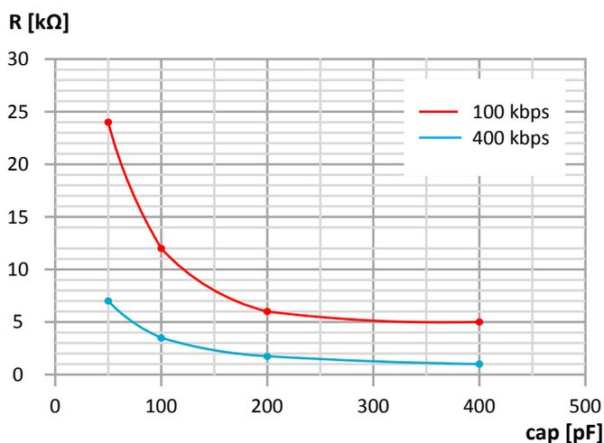
Figure 180: Recommended TWIM pullup value vs. line capacitance
