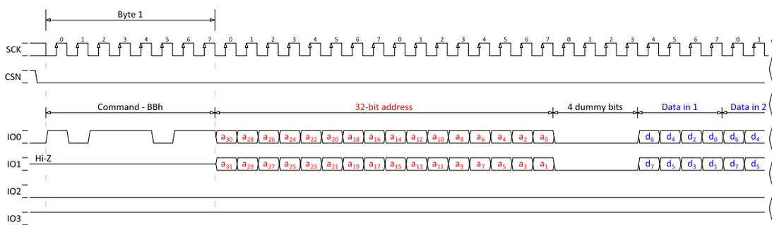
Figure 100: 32-bit READ2IO (dual read input/output), SPIMODE = MODE0
