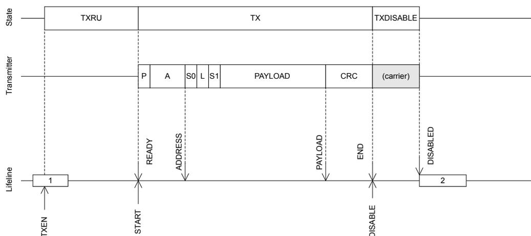
Figure 114: Transmit sequence using shortcuts to avoid delays
