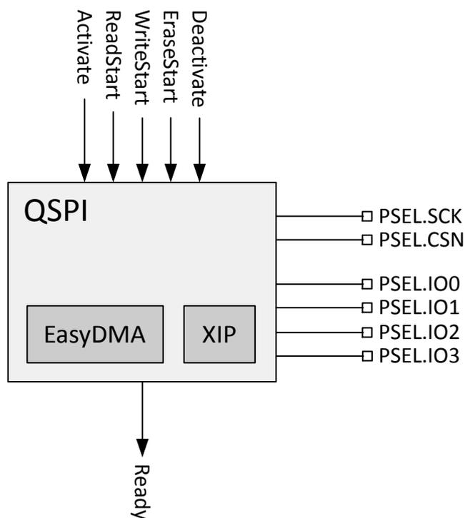
Figure 86: Block diagram
