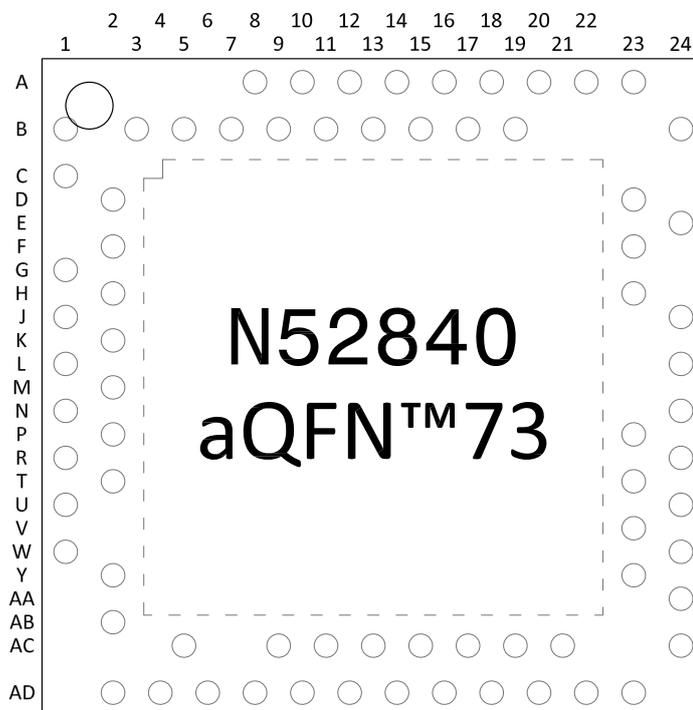
Figure 207: aQFN<sup>™</sup>73 ball assignments, top view
