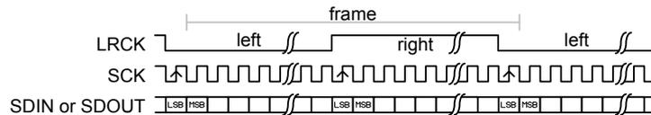
Figure 50: I<sup>2</sup>S format. CONFIG.SWIDTH equalling half-frame size.
