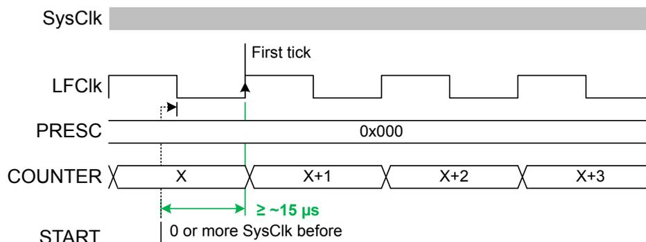
Figure 145: Timing diagram - JITTER\_START-
