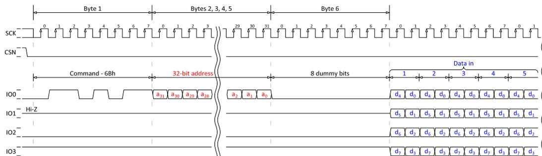
Figure 101: 32-bit READ4O (quad-read output), SPIMODE = MODE0
