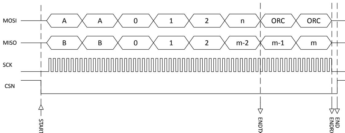
Figure 159: SPI master transaction
