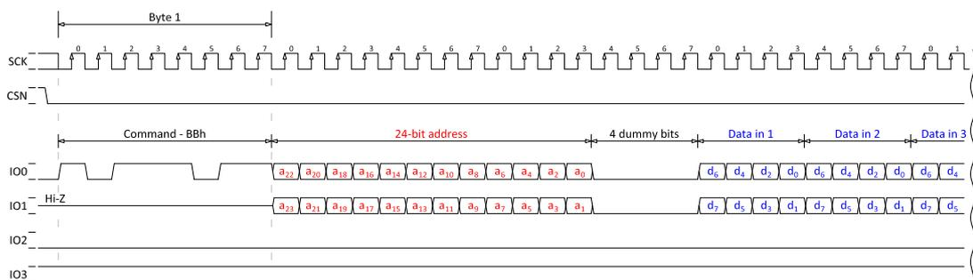
Figure 91: 24-bit READ2IO (dual read input/output), SPIMODE = MODE0
