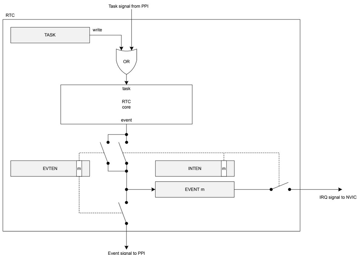
Figure 136: Tasks, events, and interrupts in the RTC
