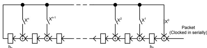
Figure 111: CRC generation of an n bit CRC
