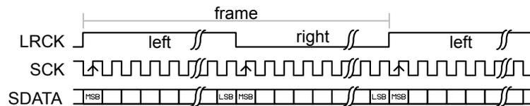
Figure 51: Aligned format. CONFIG.SWIDTH equalling half-frame size.
