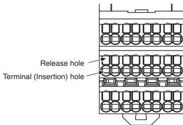
**Connecting Wires with Ferrules and Solid Wires**
