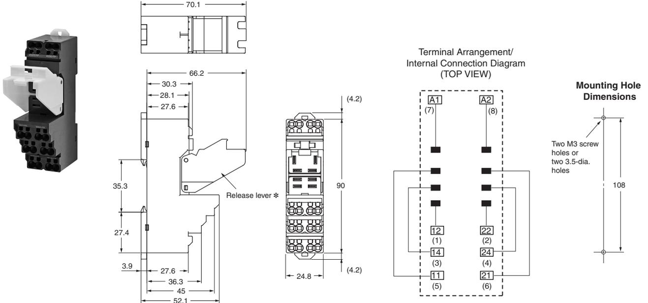
**Note:** When you apply a minimum of 10 A of current to an LY1 when it is used in combination with the PTF-08-PU(-L), connect each of the following terminal pairs: (1) to (2), (3) to (4), and (5) to (6).
