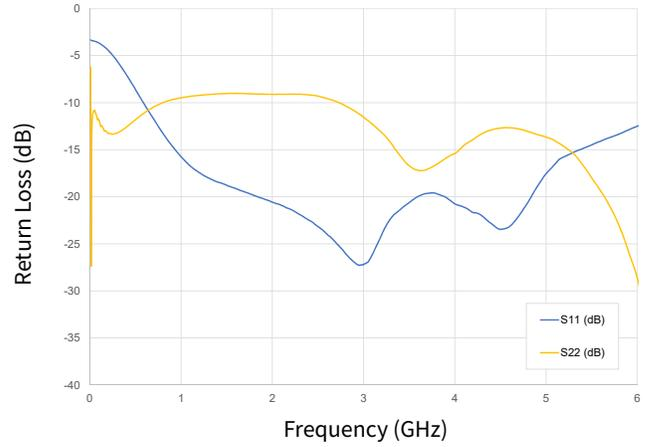
**Figure 2.** Input & Output Return Losses vs Frequency
