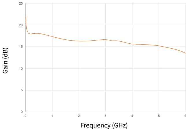
**Figure 3.** Small Signal Gain vs Frequency
