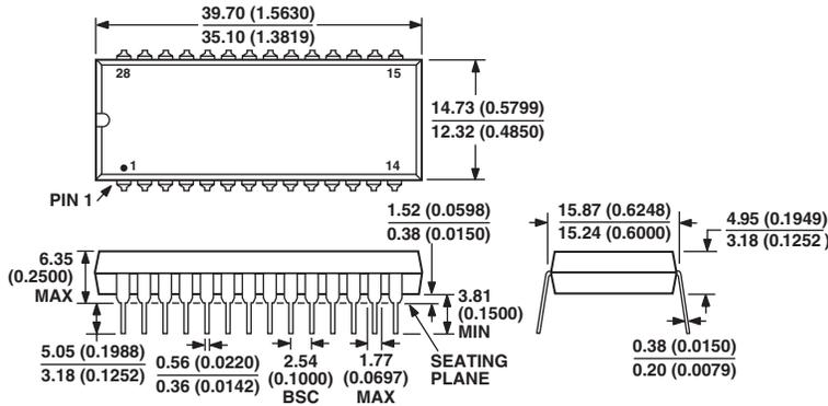
CONTROLLING DIMENSIONS ARE IN MILLIMETERS; INCH DIMENSIONS (IN PARENTHESES) ARE ROUNDED-OFF MILLIMETER EQUIVALENTS FOR REFERENCE ONLY AND ARE NOT APPROPRIATE FOR USE IN DESIGN
