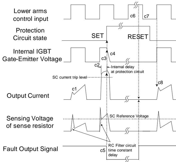
**Figure 12. Short-Circuit Current Protection (Low-Side Operation only)**
