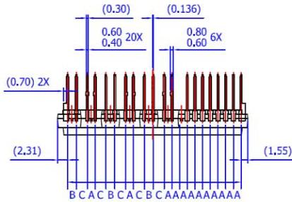
LEAD PITCH (TOLERANCE : ±0.30)
