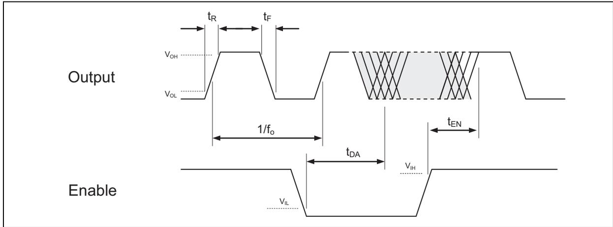
FIGURE 3-1: OE Function and Output Waveform: LVCMOS.
