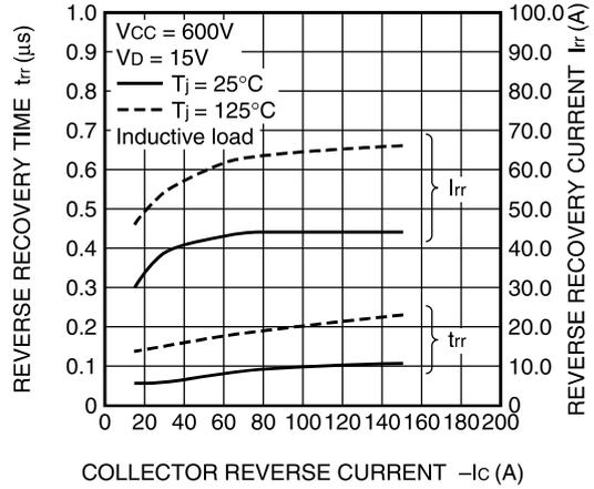
**SWITCHING RECOVERY LOSS CHARACTERISTICS (TYPICAL)**
