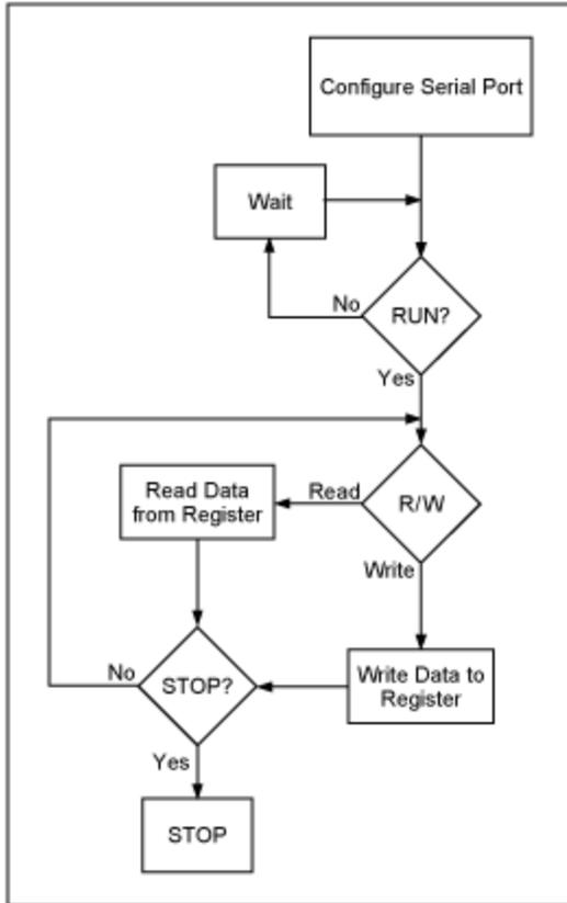
Figure 3. Communicate\_2wire.vi Flow Chart.
