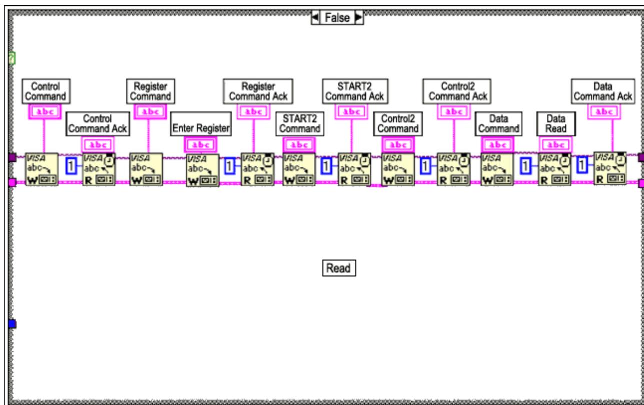
Figure 8. Serial Read. After the write or read is completed, the program waits for the user to write or read another register or stop the program. If the STOP button is clicked, the program will stop even if it is not finished writing to the 2-wire device.
