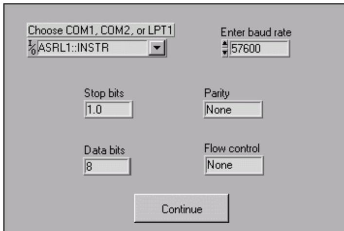
Figure 4. Enter Serial Port Settings Front Panel.
