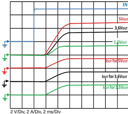
**Fig. 22 - Typical Turn-On Delay, Rise Time**
