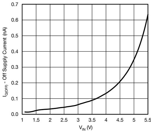
**Fig. 5 - Off Supply Current vs. Input Voltage**
