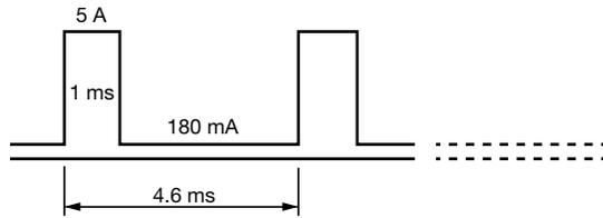
The SiP32508 and SiP32509 can safely support 5 A pulse current repetitively at 25 °C.
