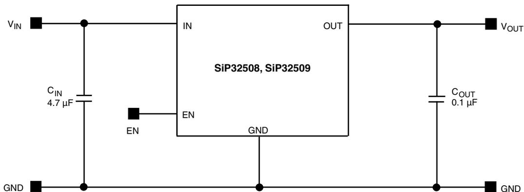
Fig. 1 - SiP32508, SiP32509 Typical Application Circuit
