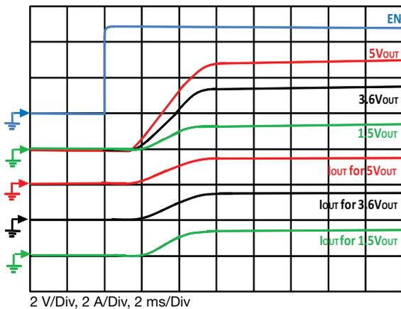
Fig. 19 - Typical Turn-On Delay, Rise Time
