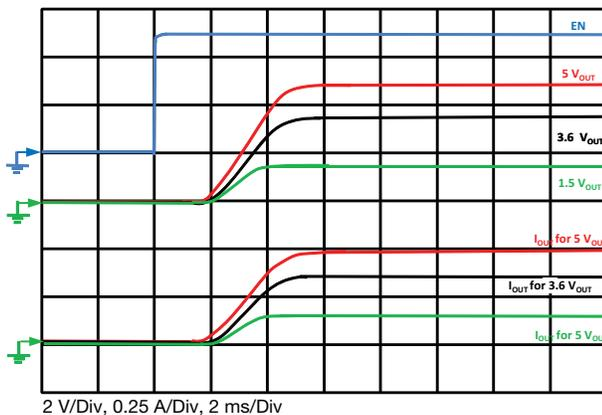
**Fig. 23 - Typical Turn-On Delay, Rise Time**
