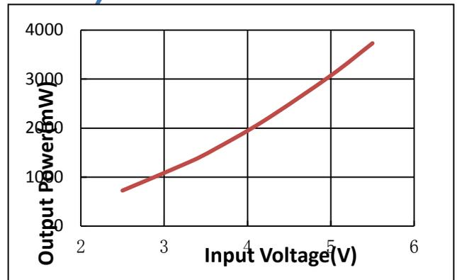
**Performance Characteristics** (@ $T_A = +25^\circ\text{C}$ ,  $V_{DD} = 5\text{V}$ , Gain = 24dB,  $R_L = L(33\mu\text{H}) + R + L(33\mu\text{H})$ , unless otherwise noted.)
