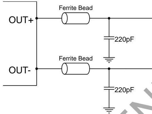
Figure 3: Ferrite Bead Filter to reduce EMI
