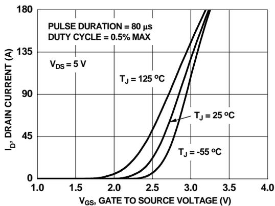
**Figure 5. Transfer Characteristics**
