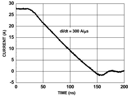
Figure 14. FDMS7570S SyncFET body diode reverse recovery characteristic
