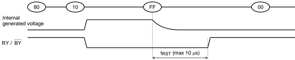
When a Reset (FFh) command is input during Erase operation
