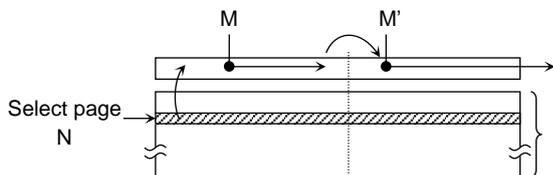
During the serial data output from the register, the column address can be changed by inputting a new column address using the 05h and E0h commands. The data is read out in serially starting at the new column address. Random Column Address Change operation can be done multiple times within the same page.
