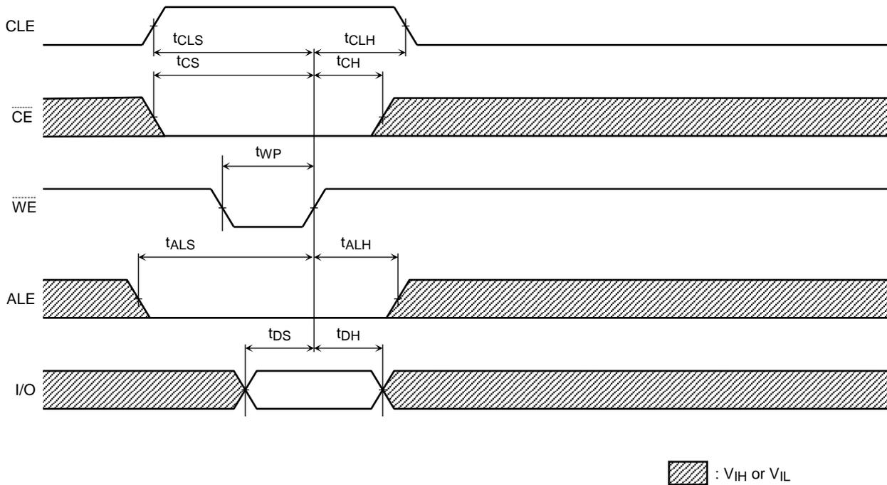
Address Input Cycle Timing Diagram
