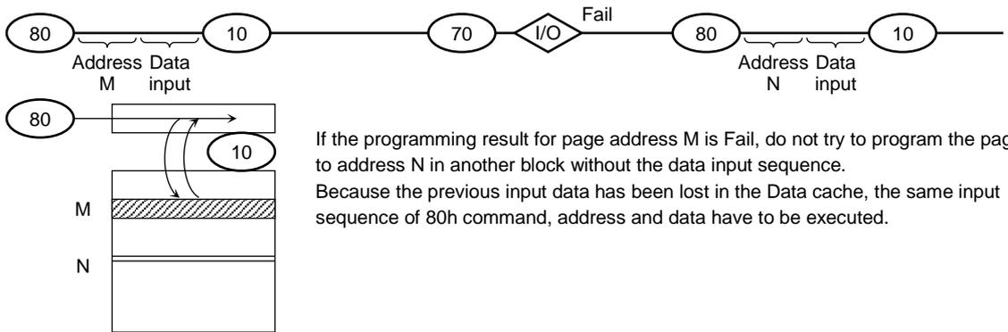
If the programming result for page address M is Fail, do not try to program the page to address N in another block without the data input sequence. Because the previous input data has been lost in the Data cache, the same input sequence of 80h command, address and data have to be executed.
