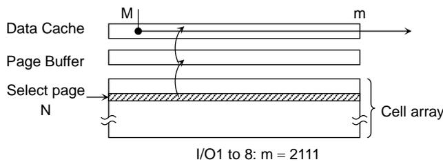
A data transfer operation from the cell array to the Data Cache via Page Buffer starts on the rising edge of WE in the 30h command input cycle (after the address information has been latched). The device will be in the Busy state during this transfer period.
