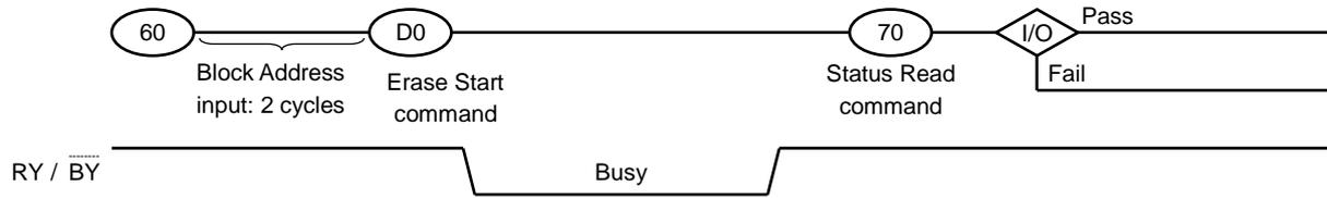
**READ FOR COPY-BACK WITH DATA OUTPUT TIMING GUIDE**
