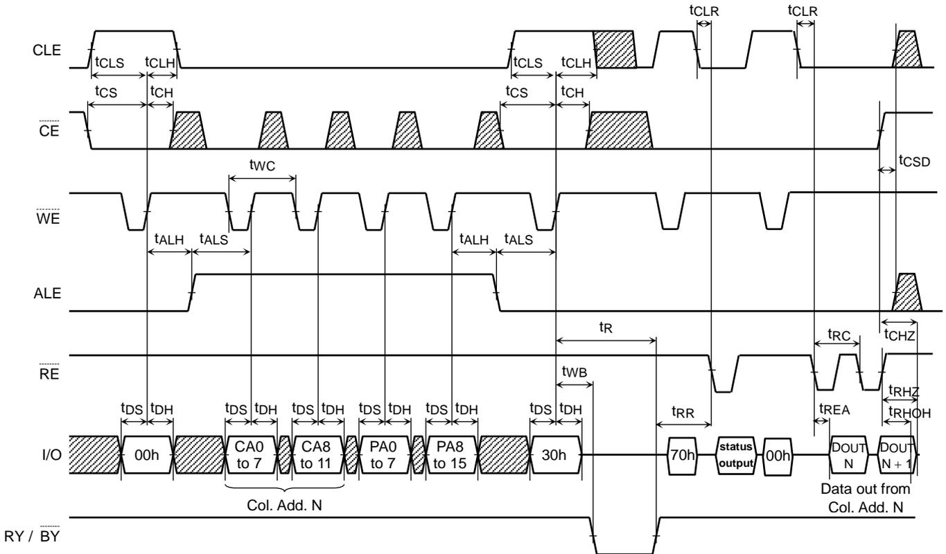
Column Address Change in Read Cycle Timing Diagram (1/2)
