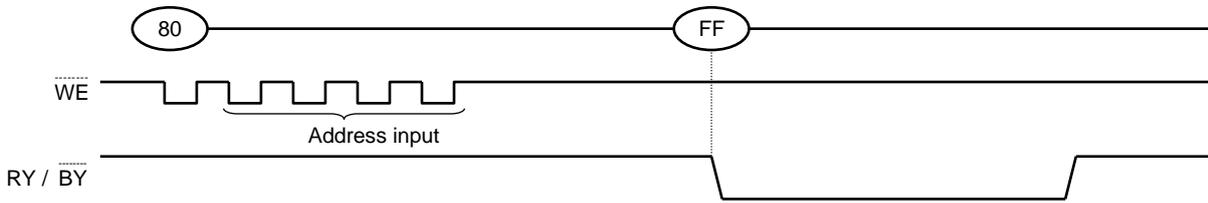
If a command other than "85h", "10h" or "FFh" is input, the Program operation is not performed and the device operation is set to the mode that the input command specifies.
