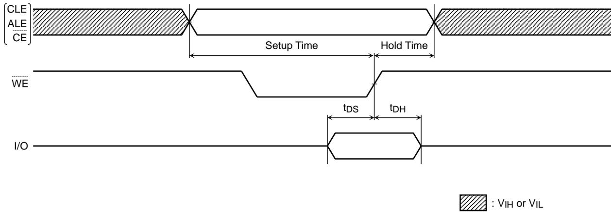
Command Input Cycle Timing Diagram
