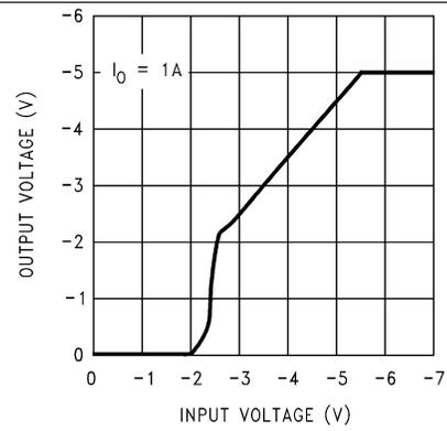
Figure 6. LM2990-5 and LM2990-5.2 Low Voltage Behavior
