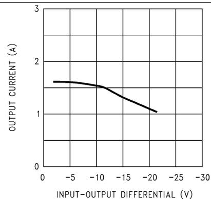
Figure 14. Maximum Output Current
