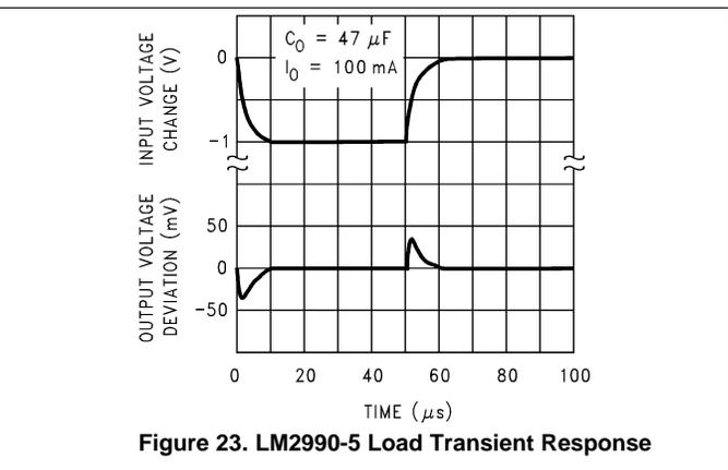
Figure 23. LM2990-5 Load Transient Response
