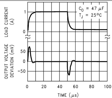
Figure 10. LM2990-12 and LM2990-15 Line Transient Response
