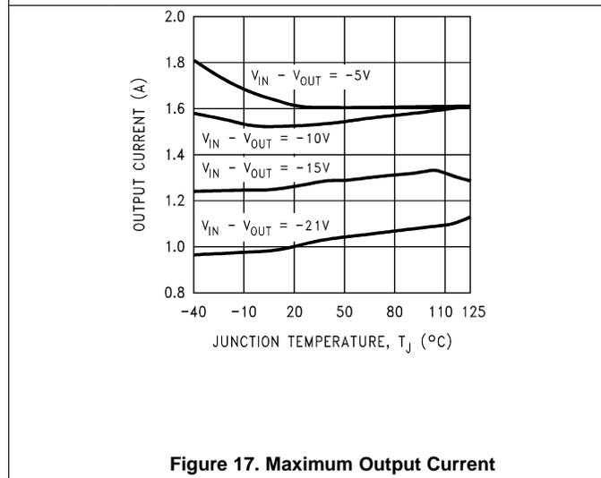
Figure 17. Maximum Output Current
