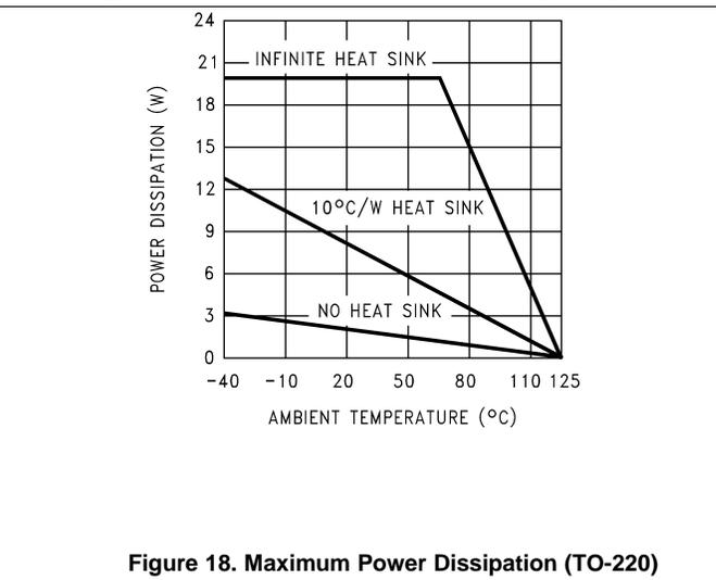
Figure 18. Maximum Power Dissipation (TO-220)
