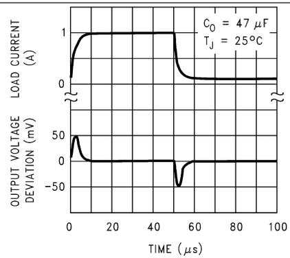
Figure 8. LM2990-5 and LM2990-5.2 Load Transient Response
