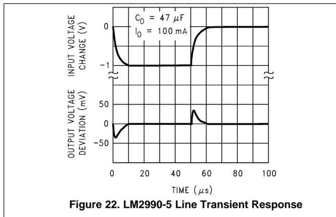
Figure 22. LM2990-5 Line Transient Response
