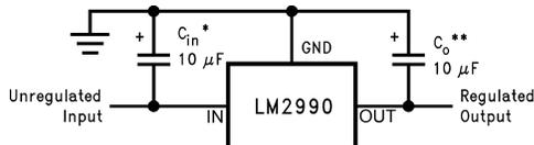
\* and \*\*: Required for stability. Must be at least a 10- $\mu\text{F}$  aluminum electrolytic or a 1- $\mu\text{F}$  solid tantalum to maintain stability. May be increased without bound to maintain regulation during transients. Locate the capacitor as close as possible to the regulator. The equivalent series resistance (ESR) is critical, and should be less than 10  $\Omega$  over the same operating temperature range as the regulator.
