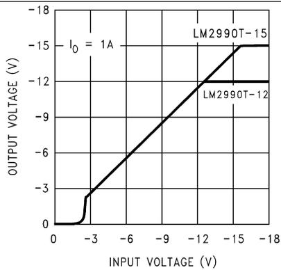
Figure 9. LM2990-12 and LM2990-15 Low-Voltage Behavior
