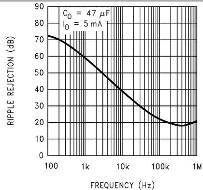
Figure 12. LM2990-5 and LM2990-5.2 Ripple Rejection
