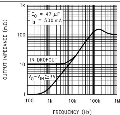
Figure 13. LM2990-5 and LM2990-5.2 Output Impedance
