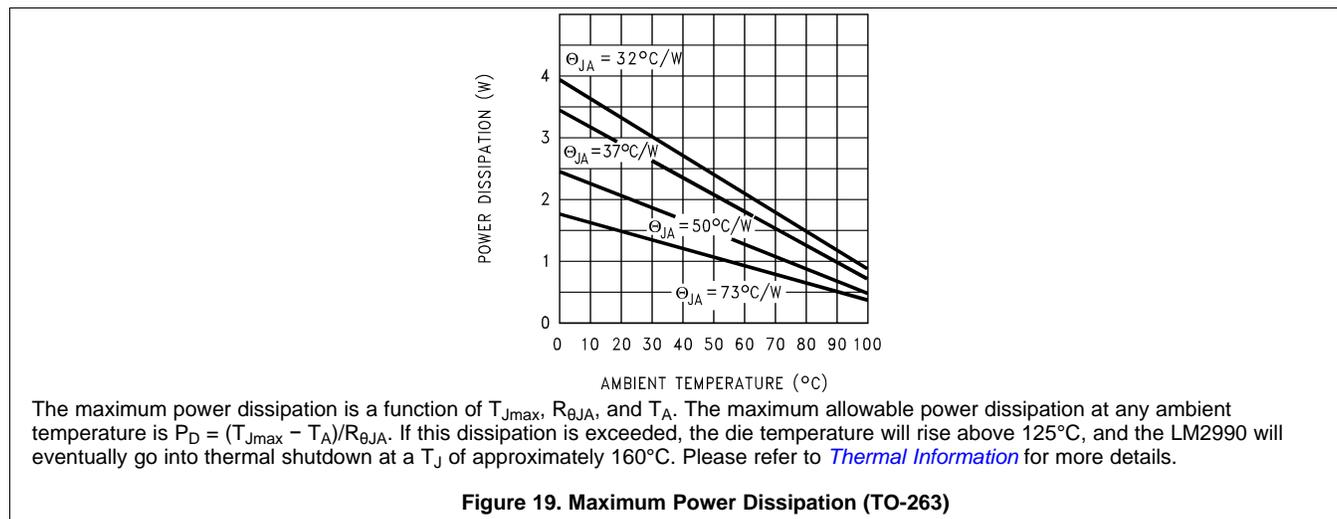
Figure 19. Maximum Power Dissipation (TO-263)
