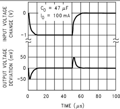
Figure 11. LM2990-12 and LM2990-15 Load Transient Response
