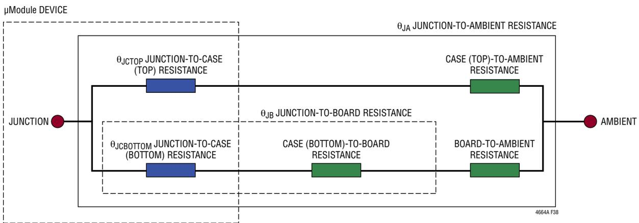
Figure 38. Graphical Representation of JESD51-12 Thermal Coefficients
