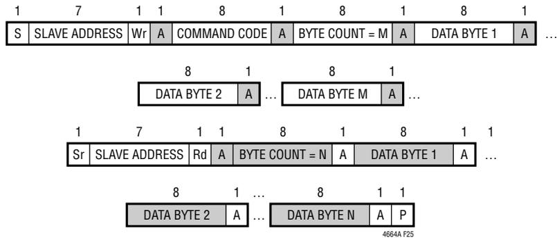
Figure 25. Block Write – Block Read Process Call
