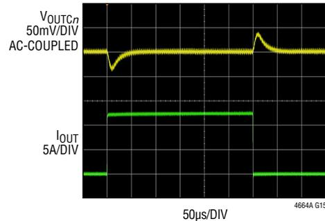
48V TO 1.5V SINGLE CHANNEL, 0A TO 12.5A/μs
