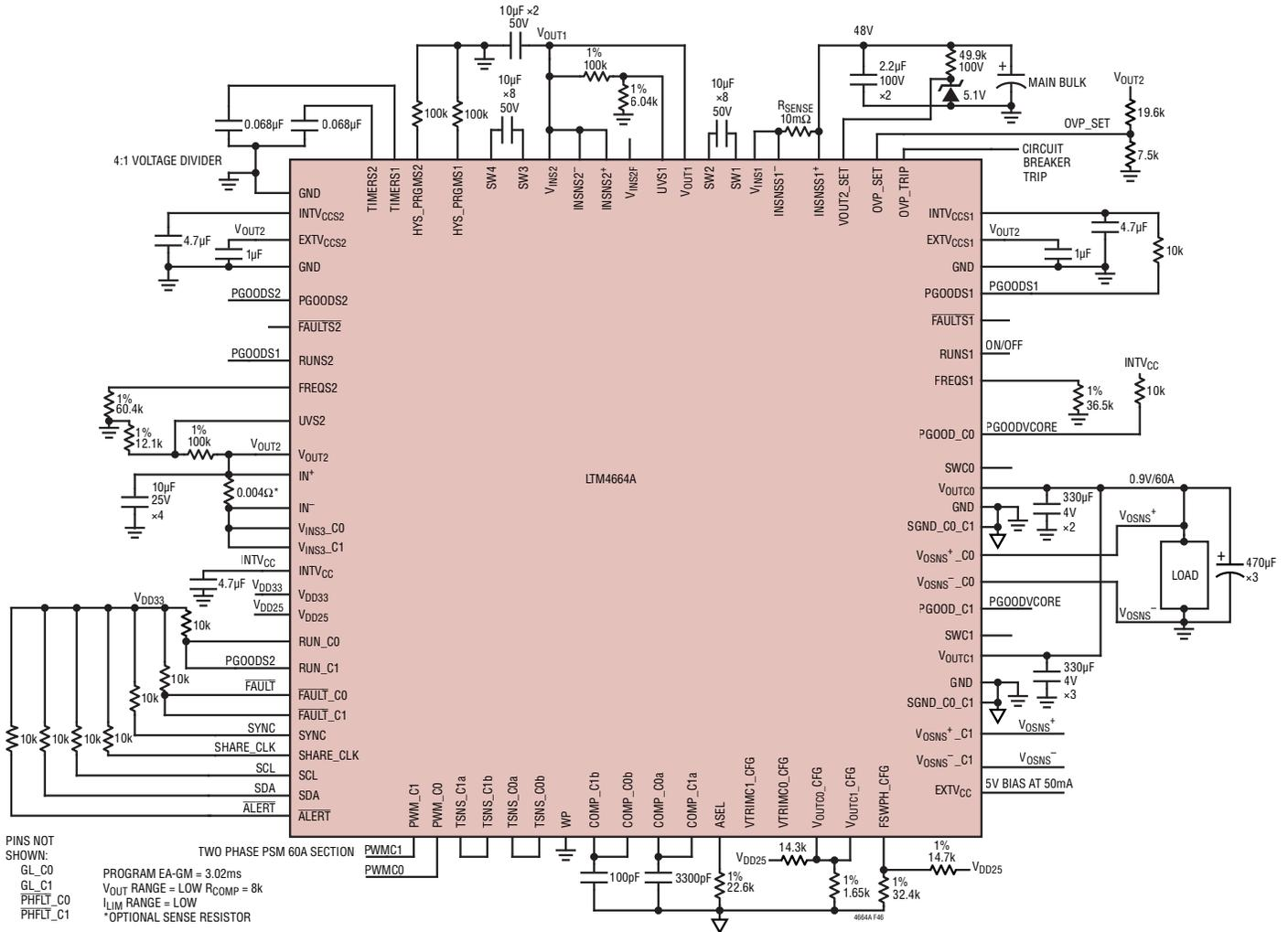
**Figure 46. 0.9V at 60A Output DC/DC  $\mu$ Module Regulator with I<sup>2</sup>C/SMBus/PMBus Serial Interface Including Hot Swap Front End with V<sub>OUT2</sub> OVP Protection**
