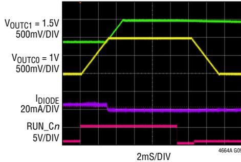
48VIN, 10A LOAD ON VOUT0, 7.5mA LOAD ON VOUT1, VOUT1 PREBIASED THROUGH A DIODE
