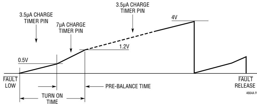
Figure 7. Timer Behavior During Fault or Startup
