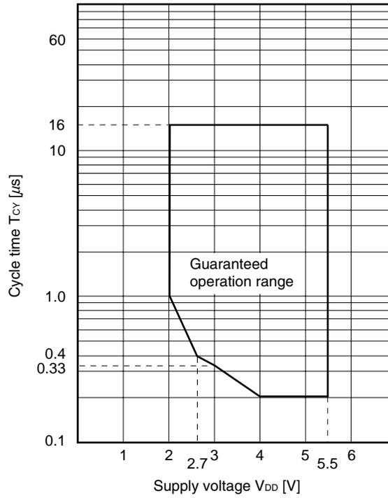
**T<sub>CY</sub> vs. V<sub>DD</sub> (High-speed internal oscillator Clock)**
