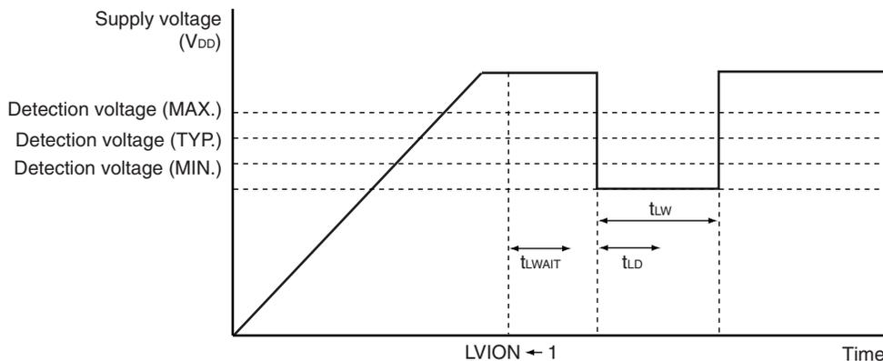
**Data Memory STOP Mode Low Supply Voltage Data Retention Characteristics (T<sub>A</sub> = -40 to +85°C)**
