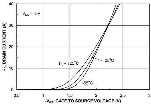
Figure 5. Transfer Characteristics.
