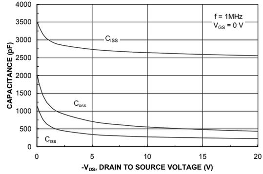
Figure 8. Capacitance Characteristics.
