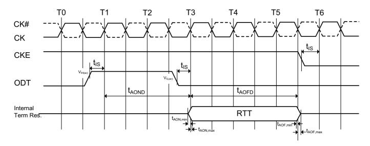
Figure 14. ODT timing for power-down mode
