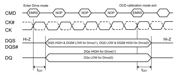
NOTE : Drive mode, both Drive(1) and Drive(0), is used for controllers to measure DDR2 SDRAM Driver impedance.In this mode, all outputs are driven out  $t_{\text{OIT}}$  after "enter drive mode" command and all output drivers are turned-off  $t_{\text{OIT}}$  after "OCD calibration mode exit" command.
