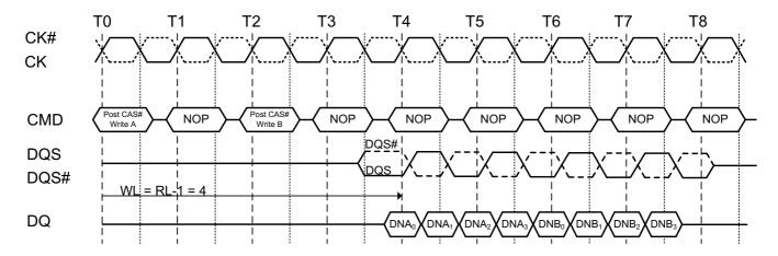
NOTE: The seamless burst write operation is supported by enabling a write command every other clock for BL= 4 operation, every four clocks for BL = 8 operation. This operation is allowed regardless of same or different banks as long as the banks are activated.
