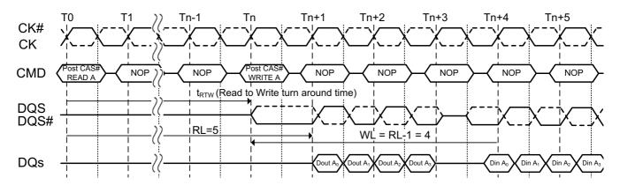
NOTE: The minimum time from the burst read command to the burst write command is defined by a read-to-write-turn-around-time, which is 4 clocks in case of BL = 4 operation, 6 clocks in case of BL = 8 operation.
