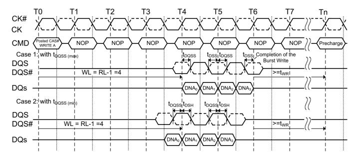
Figure 28. Burst write operation: RL=3 (AL=0, CL=3), WL=2, BL=4
