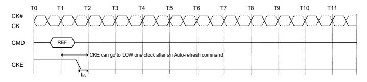
Figure 56. Active command to power-down entry
