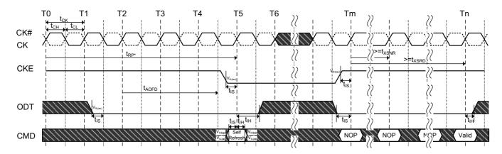
NOTE 1 Device must be in the "All banks idle" state prior to entering Self Refresh mode.
