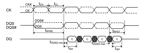
Figure 21. Data input (write) timing
