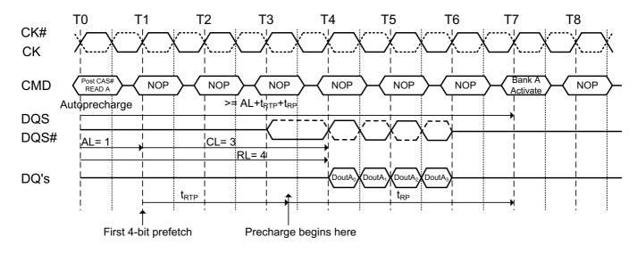
Figure 42. Burst read operation with auto precharge followed by activation to the same bank ( $t_{RC}$  Limit): RL=5(AL=2, CL=3, internal  $t_{RCD}$ =3, BL=4,  $t_{RTP}$  $\leq$ 2 clocks)
