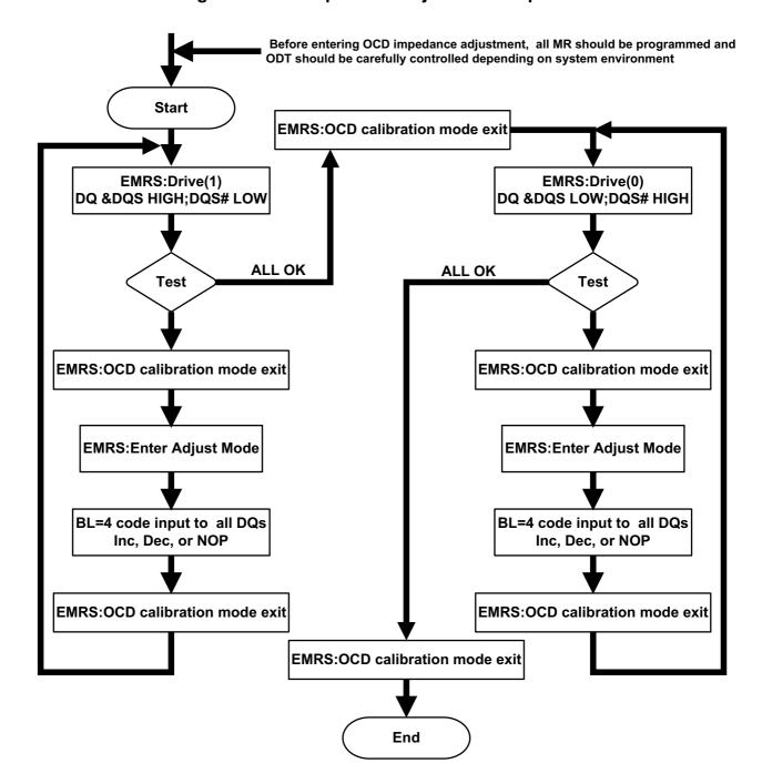
Figure 4. OCD impedance adjustment sequence
