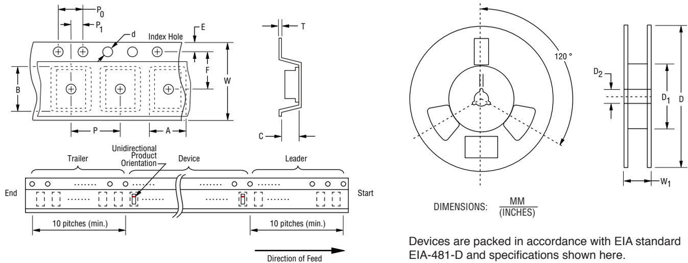
Devices are packed in accordance with EIA standard EIA-481-D and specifications shown here.
