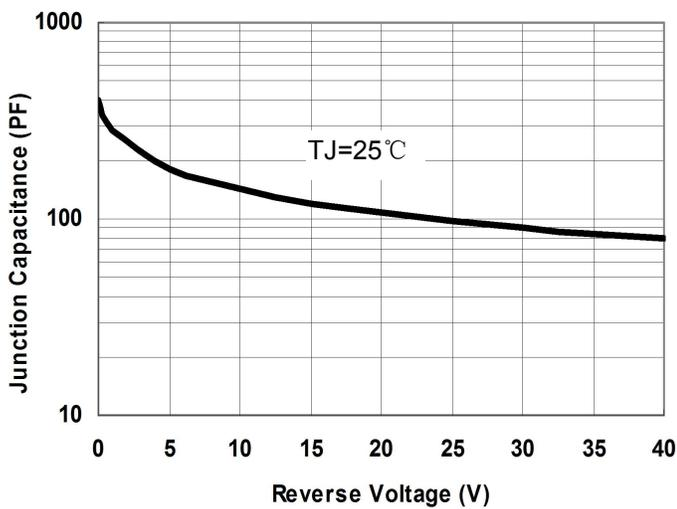
Fig.1-Typical Junction Capacitance
