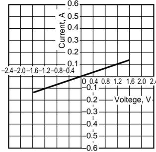
10. Off state leakage current
