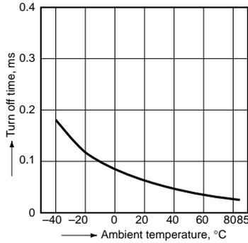
6. LED operate vs. ambient temperature characteristics
