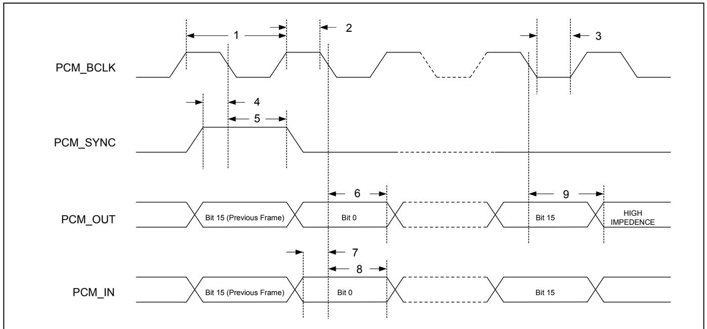
**Table 23. PCM Interface Timing Specifications (Long Frame Synchronization, Master Mode)**
