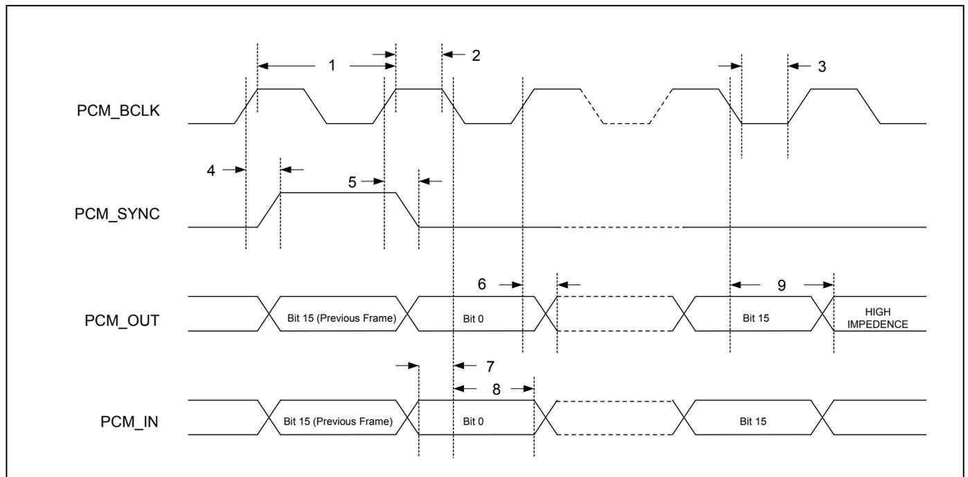
**Table 22. PCM Interface Timing Specifications (Short Frame Synchronization, Slave Mode)**
