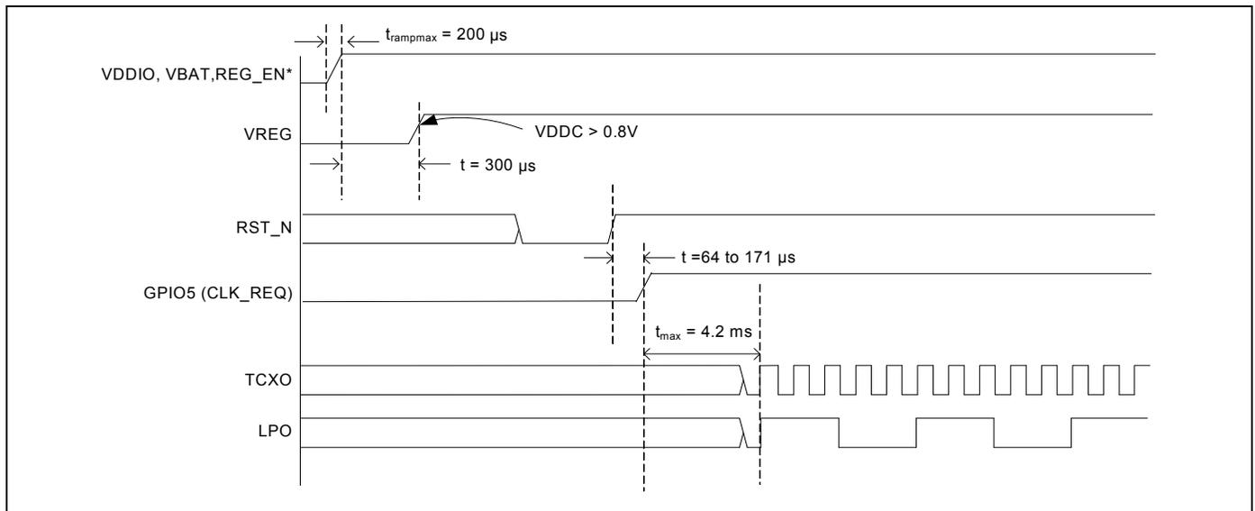
**Figure 10. Startup Timing from Power-on Reset**
