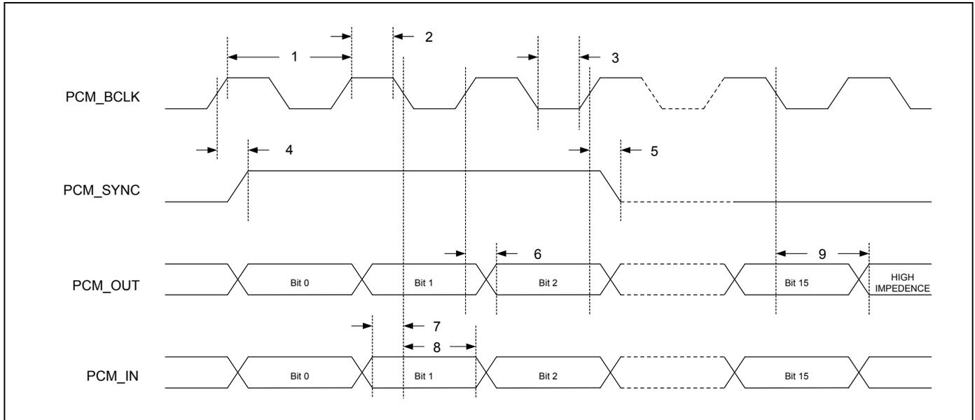
**Table 24. PCM Interface Timing Specifications (Long Frame Synchronization, Slave Mode)**
