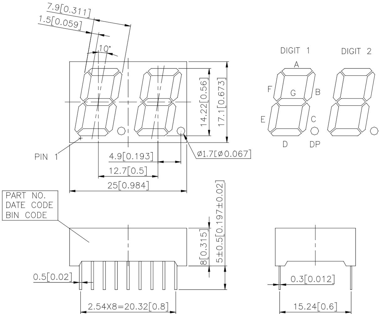
NOTES: All dimensions are in millimeters. Tolerances are ± 0.25 mm unless otherwise noted.
