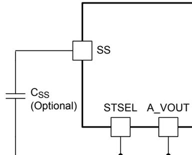
Figure 45. Slow-Start Capacitor (C<sub>SS</sub>) and STSEL Connection
