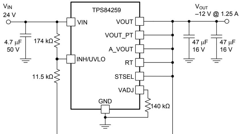
**Figure 34. Typical Schematic**
