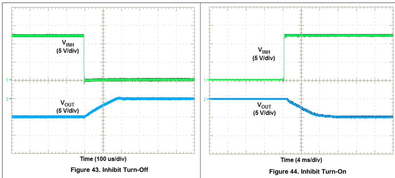
Figure 43. Inhibit Turn-Off
