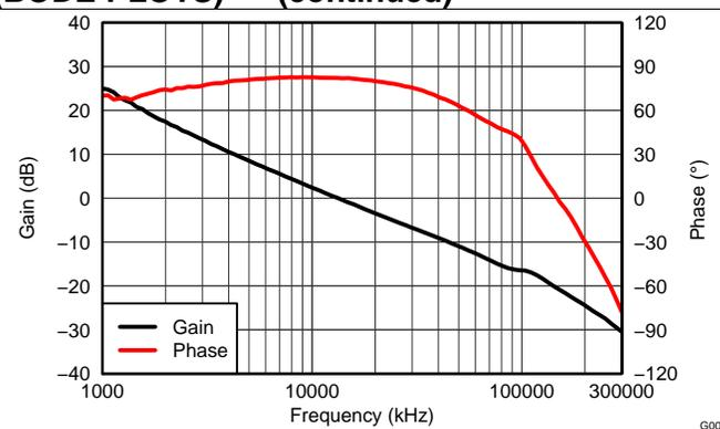
Figure 32.  $V_{IN} = 36\text{ V}$ ,  $V_{OUT} = -12\text{ V}$ ,  $I_{OUT} = 1.8\text{ A}$ ,
